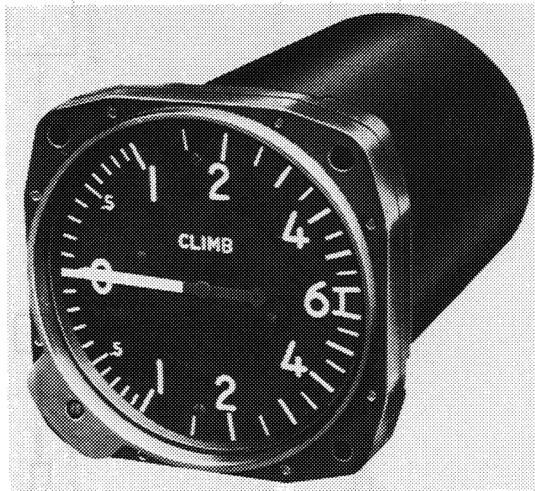
Figure 11.8.- Rate-of-climb indicator. (Courtesy of Kollsman Instrument Co.)
