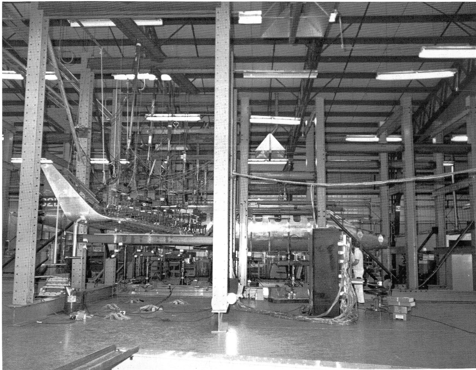
FIGURE 10 - MODEL 28/29 WING STATIC TEST SET-UP
