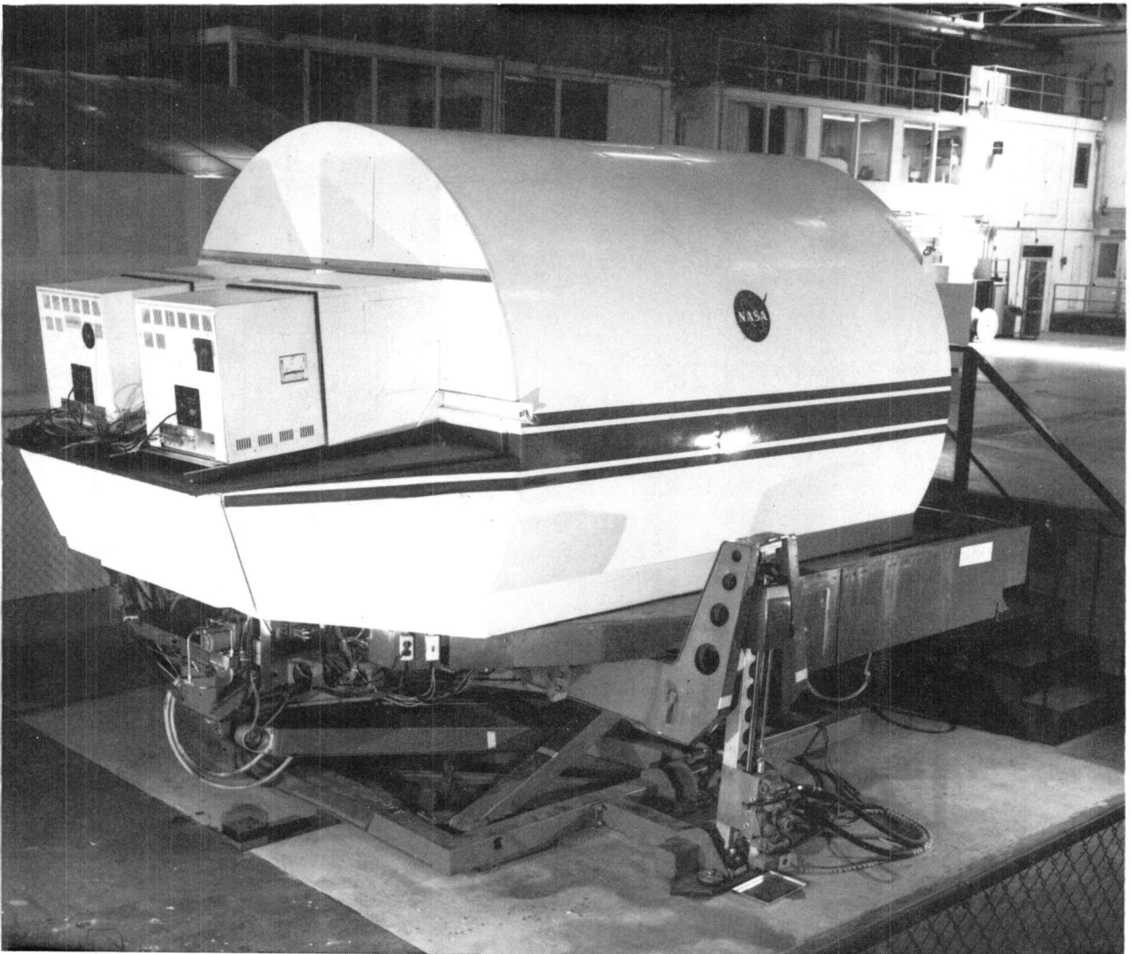
Figure 2.— Photograph of motion-base simulator used.
