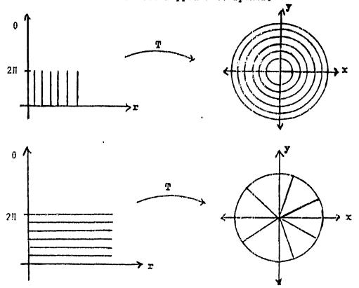
We shall consider different types of curvilinear coordinate systems by defining r and  $\theta$  as functions of  $\xi$  and  $\eta$ . Define S as a one-to-one mapping of  $1 \le \xi \le N$ ,  $2 \le \eta \le M$  onto  $1 \le r \le 10$ ,  $0 \le \theta \le 2N$ .
