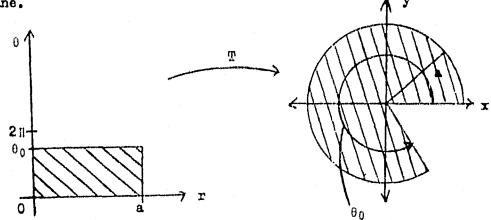
The level lines r = constant are mapped onto circles in the xy-plane and the lines n = constant are mapped onto spokes.
