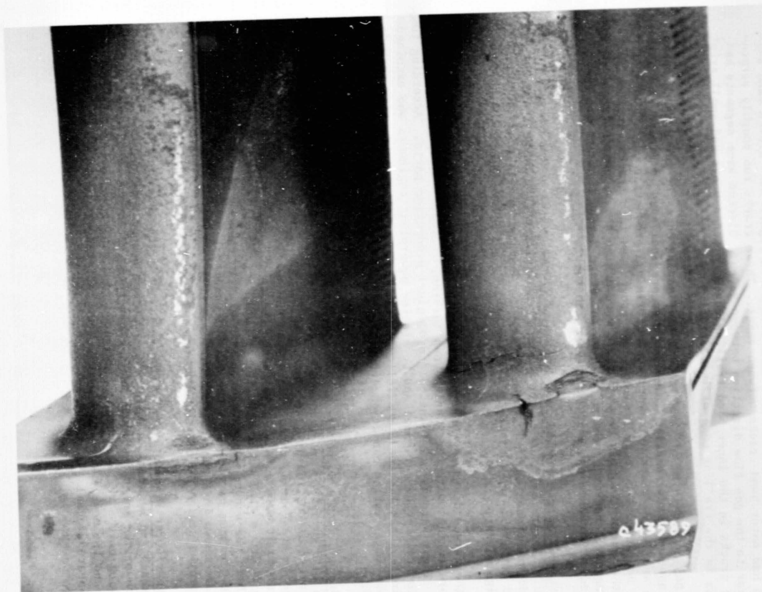
Figure 91. Stage 2 Vane Suction Side Crack After 1000 Cycles.
