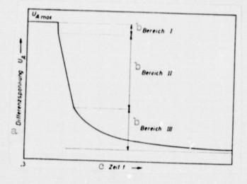
Figure 3: Schematic curve representation in the optical impregnation and wetting measurement.
