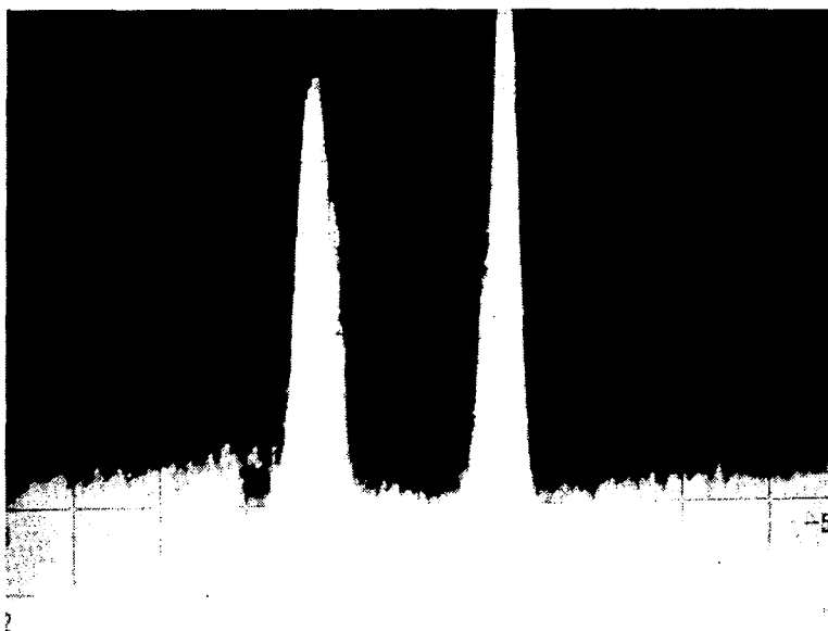
Figure 1.- Gain profile splitting due to velocity selective pumping: \text{CH}_3\text{F} pumped with 9P20 line at 3m Torr pressure; center frequency 604 GHz, 1 MHz/div.
