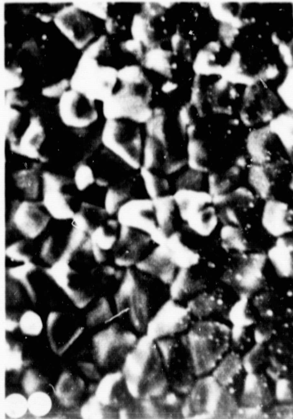
#17 Atypical As/Se Glass Surface Figure 22 S.E.M. X575
