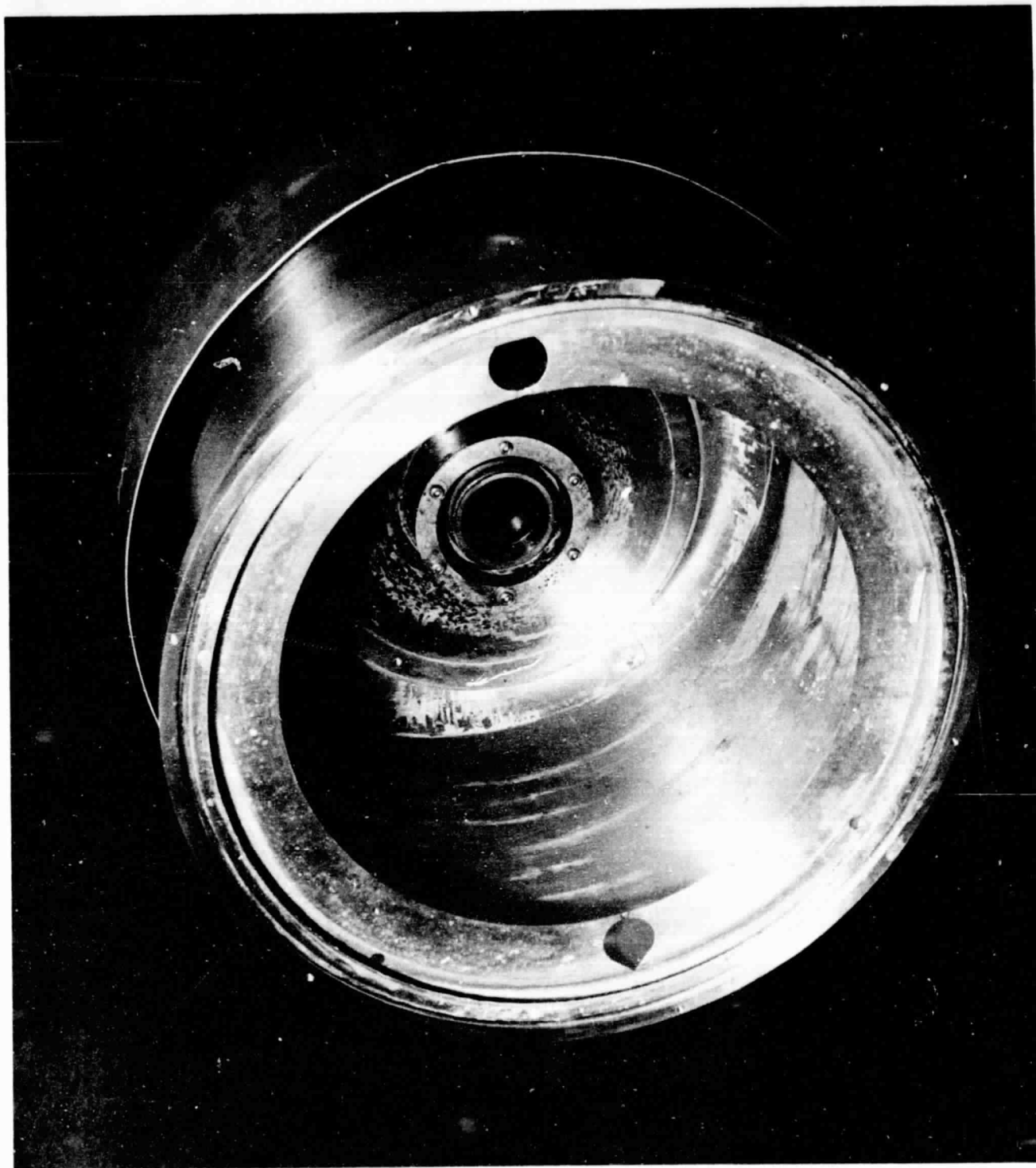
Figure 5-10 Boiler, Condenser, Desuperheater Condition after Baseline Testing
