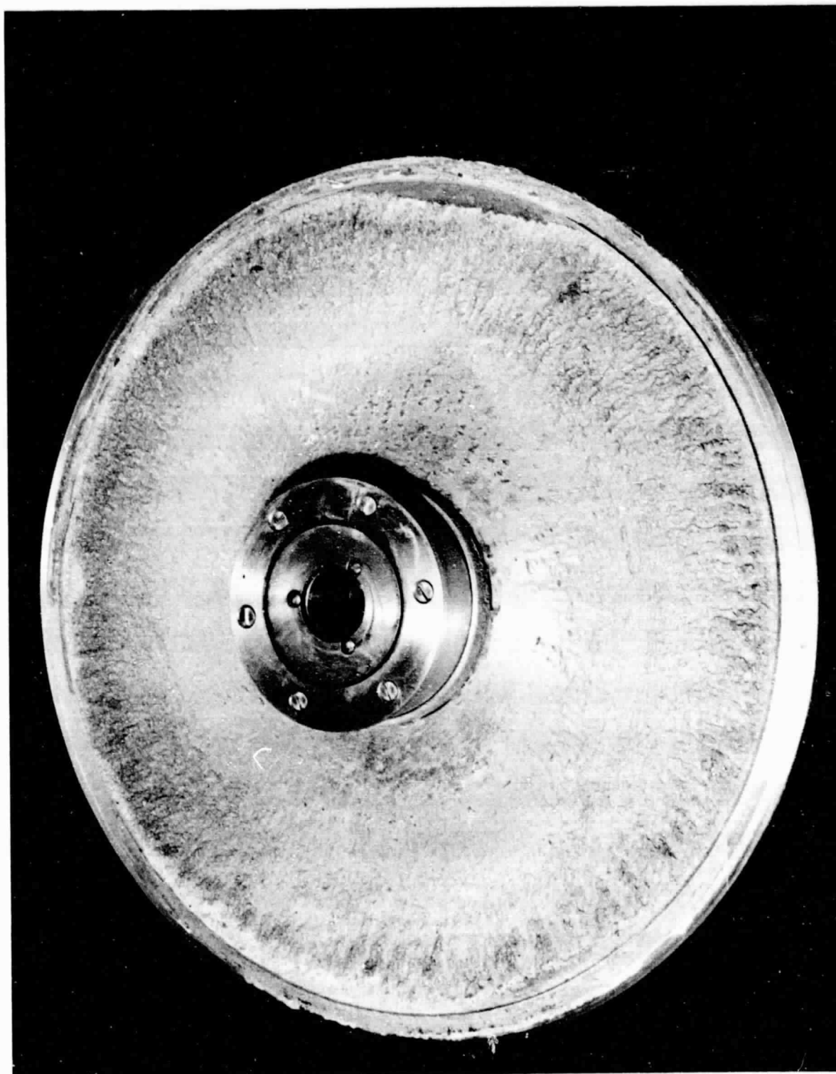
Figure 5-7 Recycle Closure Plate Condition After Baseline Testing
