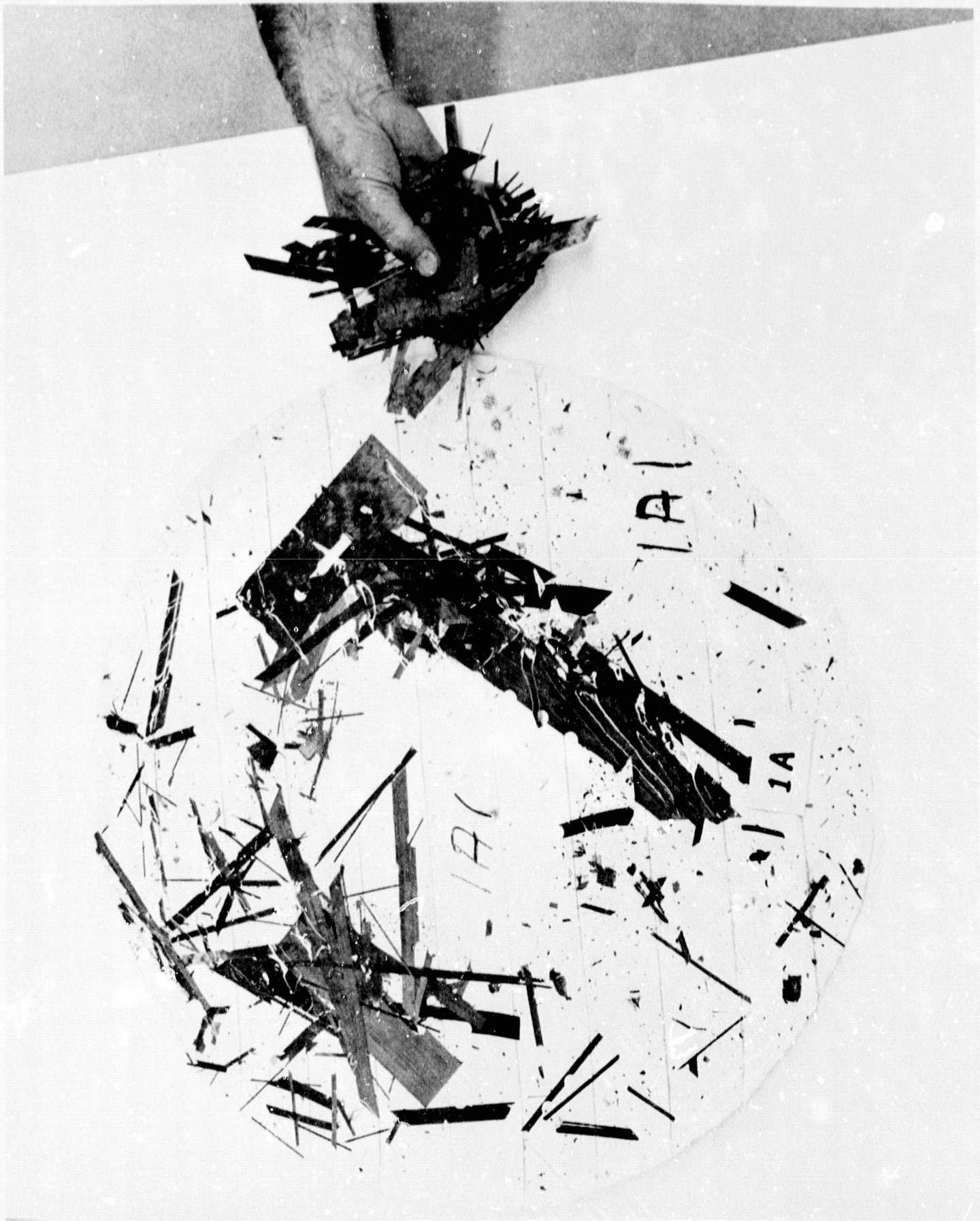
Figure 55 Hybrid System #1a After Burn, Impact, and Air Flow Test
