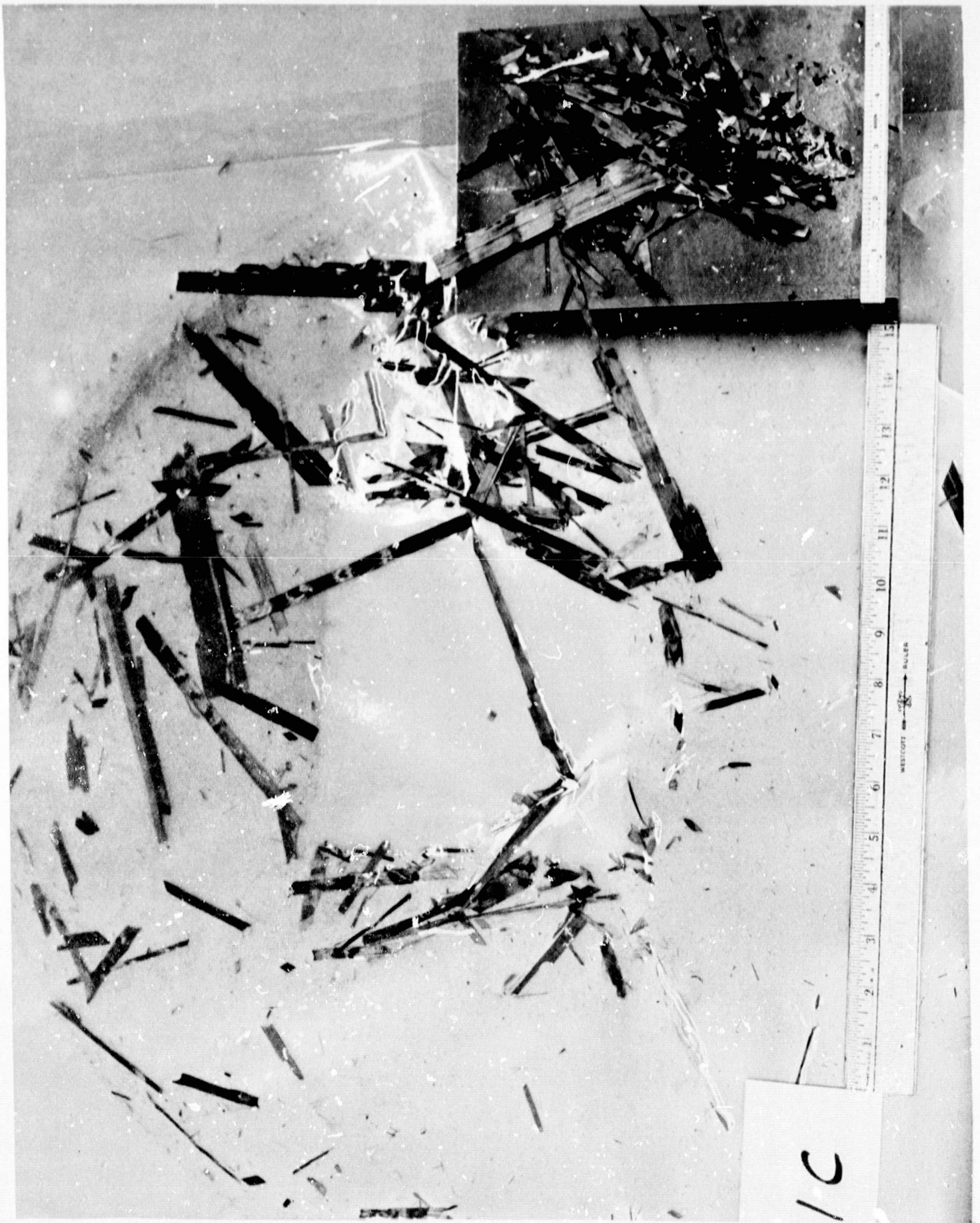
Figure 57 Hybrid System #1c After Burn, Impact, and Air Flow Test
