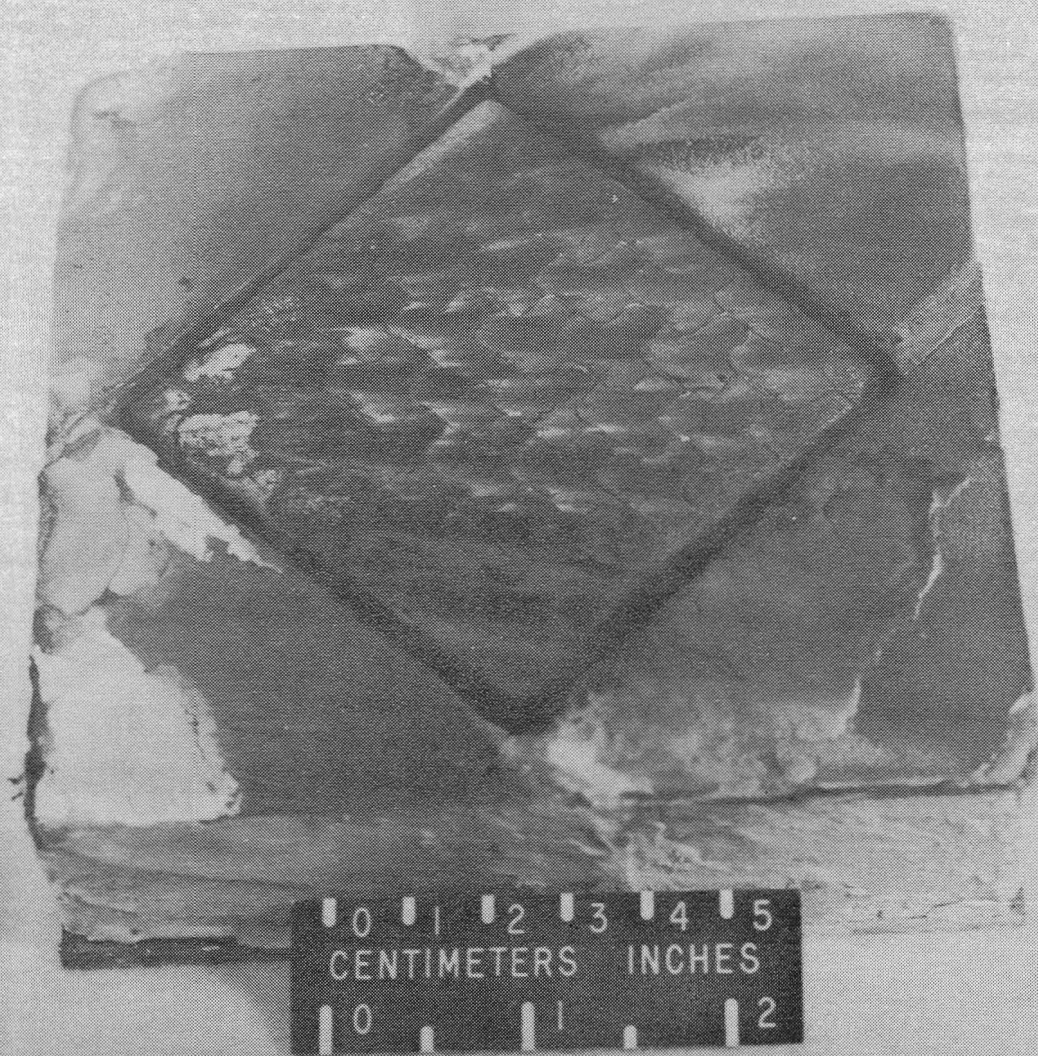
Figure 8.- Panel no. 4, SLA-561 after 450s entry test at 20 Btu/ft 2 s.
