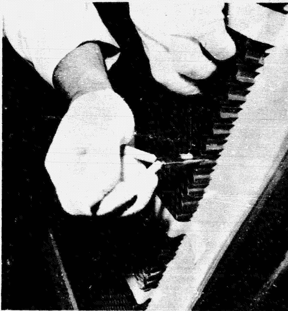
Figure 36.- Perforating honeycomb core at cell node points.
