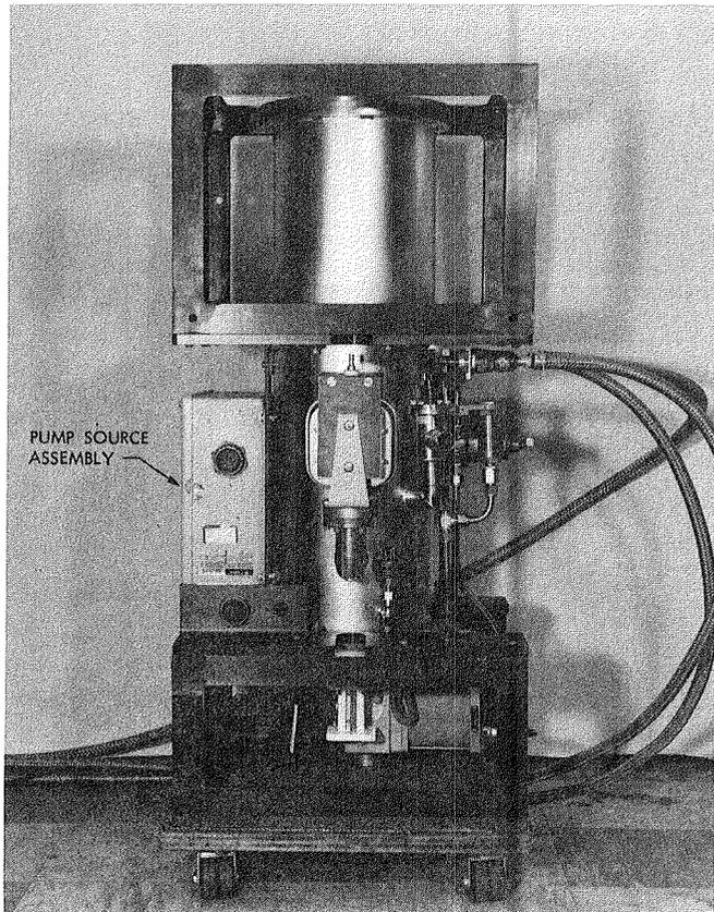
Fig. 1. X-band Block II traveling-wave maser assembly
