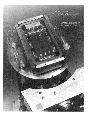
Fig. 4. X-band halfwave structure assembly mounted superconducting magnet
