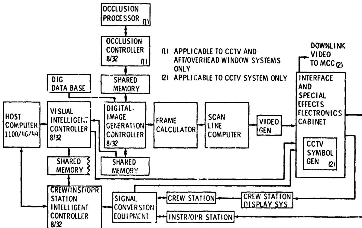
Fig. 2 SMS visual system interface.
