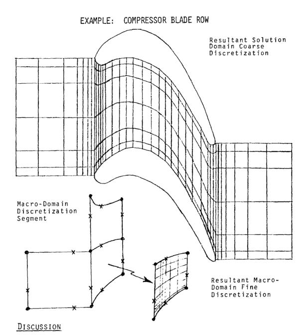
Three of the ten macro-domains, used to form the blade row discretization, are shown. The non-midside location of non-vertex nodes produces the non-uniform grid, only a few gridlines of which are shown. The inset illustrates a fine discretization of one macro-domain. The coordinates of all nodes on boundaries of macro-domains are unique.
