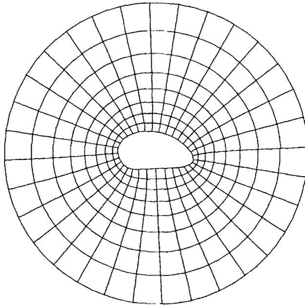
Fig. 8. Optimum mesh system - cylinder of irregular shape.
