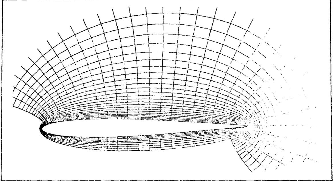
This grid has been used in a computation of a flow past a 9 % thick symmetric airfoil at an angle of attack of 15%. The grid is a bilinear grid with  $\alpha = 16$ . In this study, the boundary layer region of the flow is computed separately from the detached region. It is only necessary to generate a grid covering the computation field and to keep the singular point away from this computation field.
