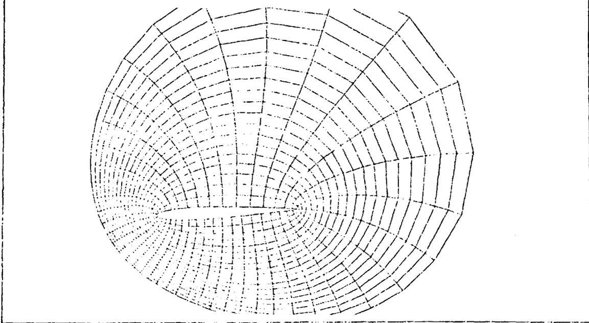
Using a complex value for  $\alpha$ , the concentric circles and radial lines in the  $w$ -plane are mapped onto non-symmetric grid lines in the airfoil-plane. The figure above shows grid lines for the case  $\alpha = \frac{1+i}{4\sqrt{2}}$ . The singular points of the grid system shown here and in the previous figure are sufficiently far from the airfoil so that the grids are of practical interest.
