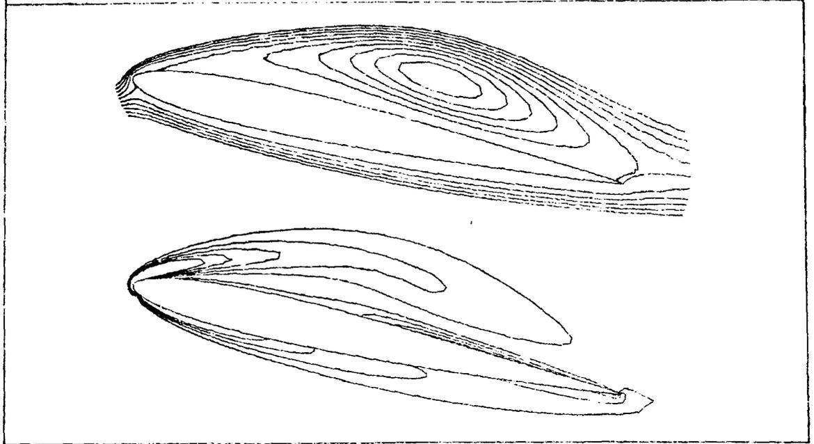
This figure shows the computed streamlines and constant vorticity contours around the airfoil after the airfoil has advanced 2.9 chord lengths relative to the freestream. A separation bubble has appeared and grown to its present size. The vorticity field is still confined to the region near the airfoil as shown. With the integro-differential approach used here, it is only necessary to perform computations in the vortical region. Therefore the grid needs only be generated for the vortical region.
