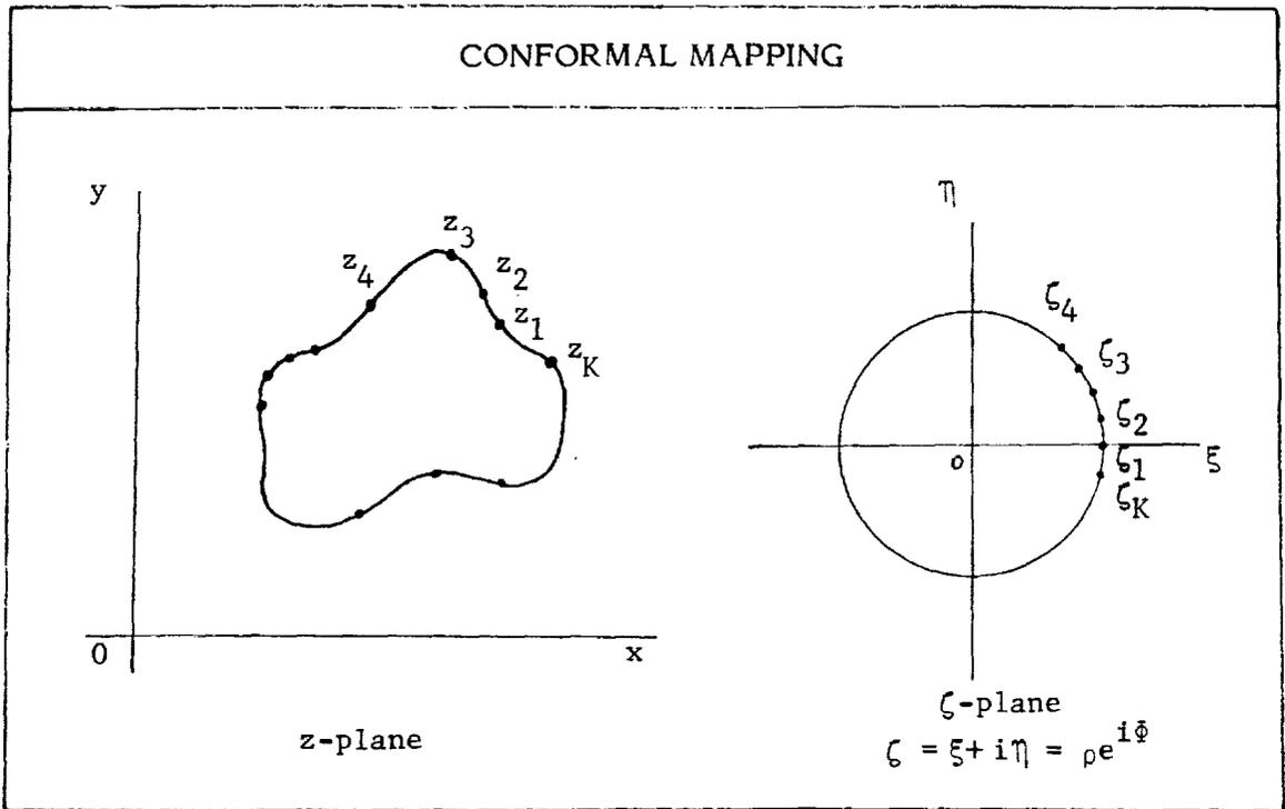
Any usual contour, open or closed, can be mapped conformally onto a simple contour, such as a circle or a straight line segment, using any prescribed distribution of the scale factor of transformation on the contour. This is true for smooth contours as well as for contours with discontinuous slopes. The unit circle is used as the canonical contour for the following discussion. A total of  $K$  equally spaced points are assigned on the unit circle, with the point  $\zeta_k$  given by
