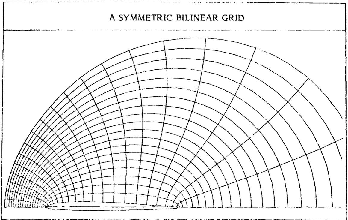
The unit circle in the  $\zeta$ -plane can be mapped onto a unit circle in the  $w$ -plane through a bilinear transformation of the form
