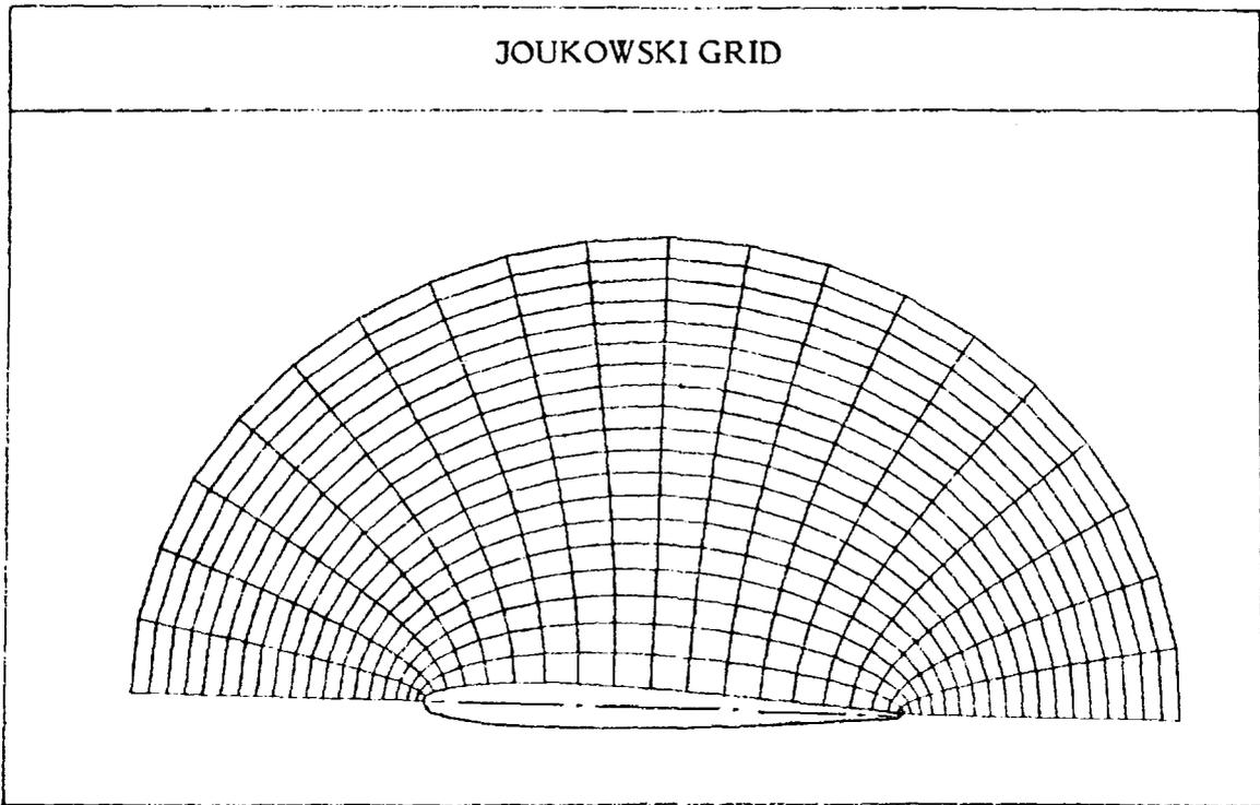
This figure shows the grid lines around a 9 % thick symmetric airfoil that is mapped using the Joukowski transformation
