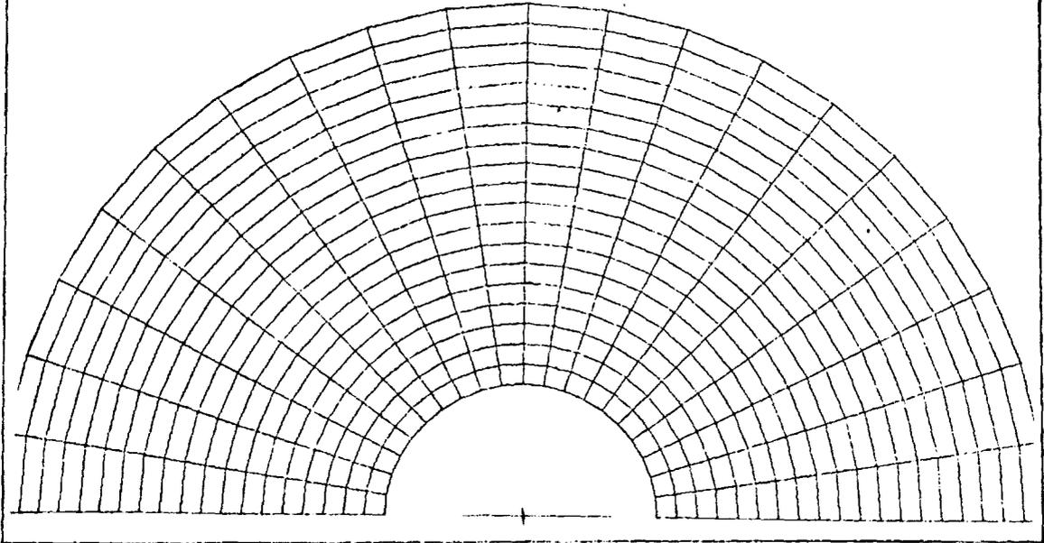
The "canonical" domain used here is the domain exterior to the unit circle. The grid lines shown here are mapped conformally onto the grid lines shown in the airfoil-planes at all points except the singular points where the mapping ceases to be conformal. The grid shown is orthogonal with equal spacings in the angular and the radial directions.
