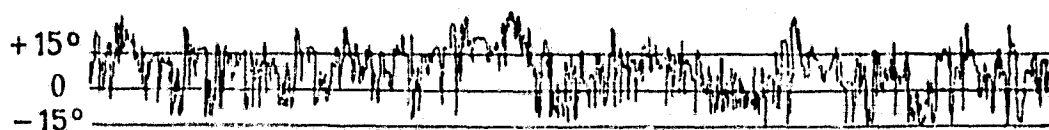
Figure 72a Instantaneous Inclination of a Sea Breeze Near the Surface of Slightly Choppy Water
