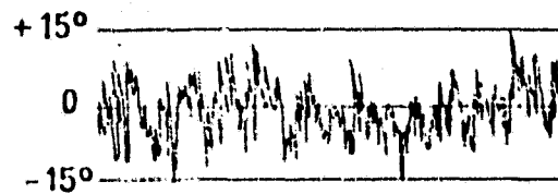
Figures 77 & 78 Inclination of a Land Breeze at Saint-Inglevert 2 m (Left) and 10 m (Right) from the Ground 1 min. = 4.7 cm
