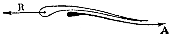
Figure 176 Propulsive Mechanism in Birds A, Flow of Air Toward the Rear B, Reaction Toward the Front
