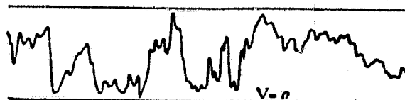
Figure 58 Speed of a NE Land Breeze Recorded at the Ile de Ré with a Hot Wire Anemometer 10 M above the Ground 1 sec = 3 mm Scale of Speed: 1.3 mm per m/sec
