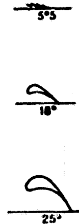
Figure 228 Soaring Albatross Wing with Cross Sections Showing Various Curvatures and Angles
