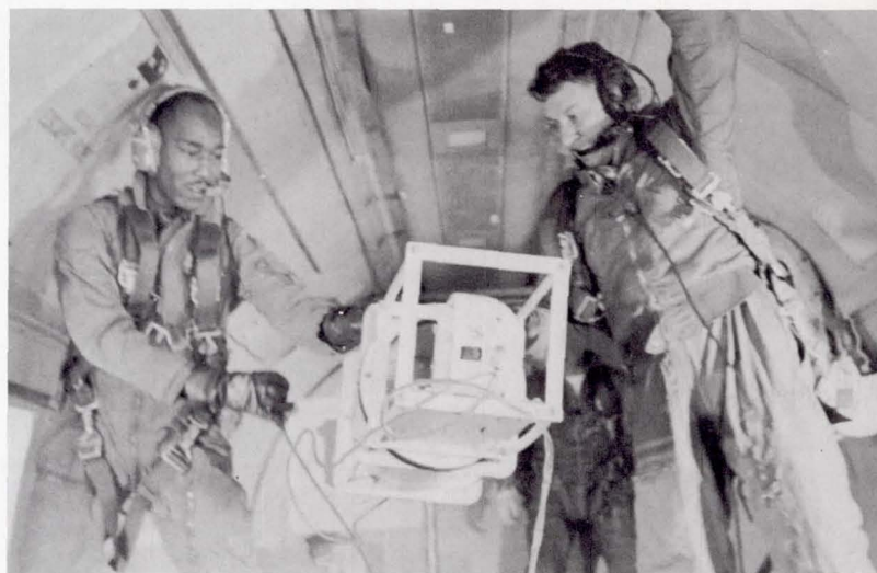
Figure 3.5. Low gravity inside a research aircraft. This photograph was taken during the reduced gravity phase of a Keplerian trajectory maneuver. The experiment package is a precursor to one of the Skylab experiments.
