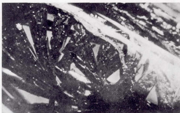
Figure 4.18. Deposition regions in GeSe ampoules processed at high transport gas pressure on Earth and in space. The most pronounced difference in growth morphology was predicted and observed for the GeSe system when the transport gas pressure was high enough to cause an extensive convective contribution to mass transport on Earth. The condensation region of the ampoule processed on Earth contains curved dendrites representative of the effect of convective turbulence on crystal habit. In the absence of convective interference on Skylab, individual well-developed crystal platelets were obtained.
