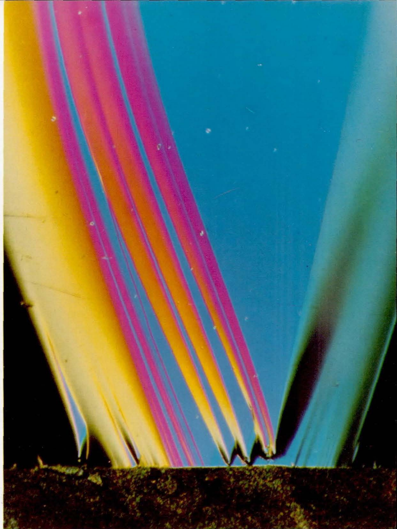
Figure 4.13. Facets on InSb crystal grown uncontained on Skylab. Facets grown on these crystals were typically flat to within a few hundred Angstrom units (1 Angstrom unit = 10^{-10} m) as may be seen by this phase contrast image. The colored lines indicate steps that appear on the curved portion of the crystal.
