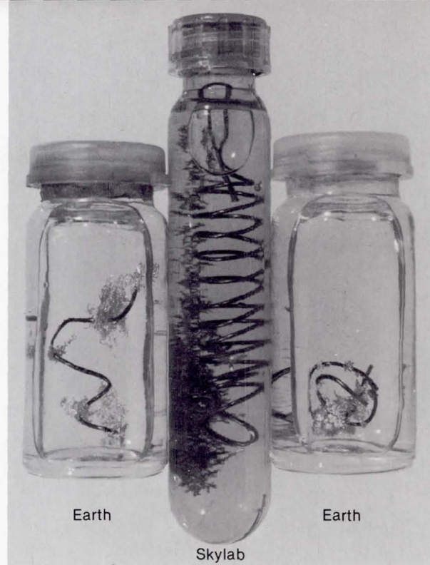
Figure 6.14. Silver crystals grown in Skylab compared with ones grown on Earth. The crystals were grown by immersing a notched copper wire in a silver nitrate solution. Silver replaced the copper at the notches. The space-grown crystals had been in the form of long filmy dendrites, which were so delicate that they broke off during handling and fell to the bottom of the vial.
