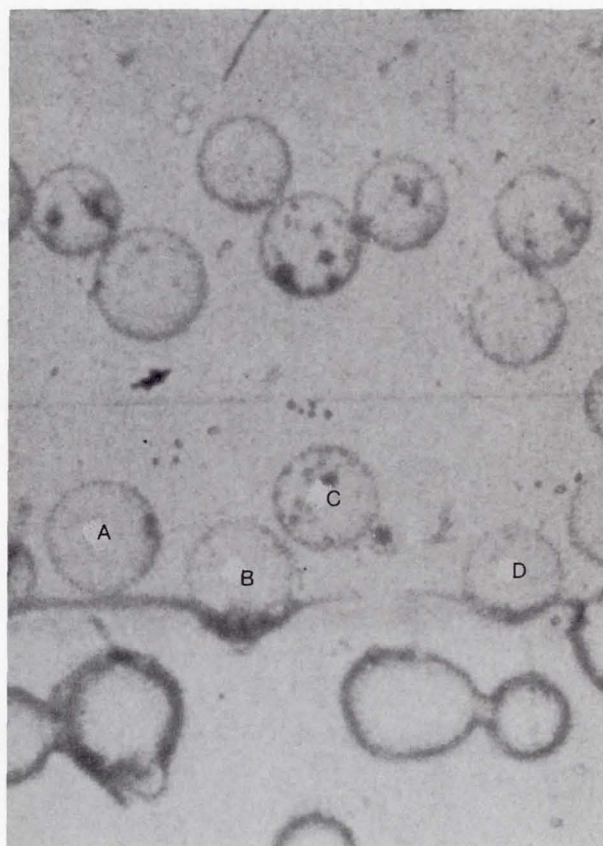
Figure 2.17. Interaction between a solidification front and second-phase particles. Glass beads ranging in size from 20 to 80\text{ }\mu\text{m} are dispersed in molten durene. The durene is being directionally solidified from bottom to top at the rate of 4.0\text{ }\mu\text{m/s} . Particles A, C, and D have been engulfed by the solidification front after being pushed a short distance. Particle B is still being pushed. Such experiments are useful in understanding the solidification of composite materials.
