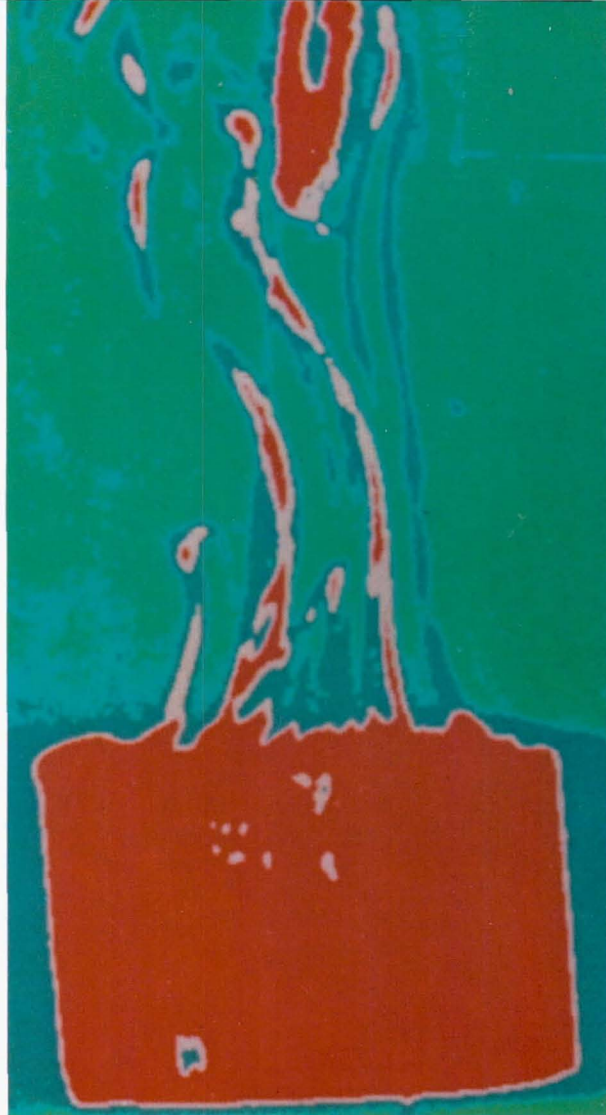
Figure 1.8. Schlieren photograph of a crystal growing from aqueous solution in Earth gravity. The convective plume is caused by the lower density of the growth solution after it has given up some of its solute to the crystal.
