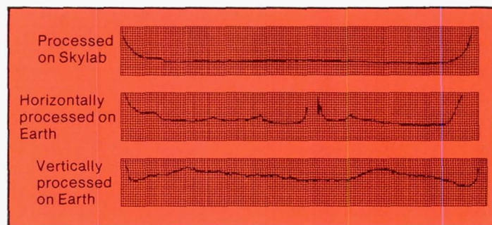
Figure 4.15. Resistivity profiles showing microsegregation in germanium. These graphs illustrate the most significant result of the experiment: influence of gravity-free solidification on microsegregation in germanium. A comparison of the resistivity profiles of three gallium-doped germanium crystals is shown. All three curves were made with the two-probe spreading resistance methods at 5\text{-}\mu\text{m} steps. The radial profiles were measured at 0.5\text{ cm} away from the original solid-liquid interface. Each unit on the horizontal axis is 100 \mu\text{m} . Microsegregation was reduced by five times and macrosegregation was reduced by six times for the Skylab processed crystal. Fluctuations in resistivity are inversely proportional to fluctuations in solute compositional variations.
