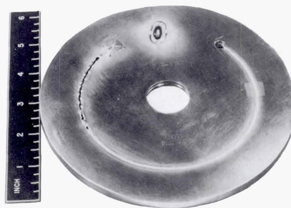
Figure 5.2. Metals melting and welding specimen after processing on Skylab. The stainless steel specimen shows the path traversed by the electron beam. The thickness varied to permit complete and partial penetration of the beam. The specimen was cut through from the 9 to 11 o'clock positions. At the 12 o'clock position, a molten puddle was formed to allow detailed studies of metal resolidification to be made.
