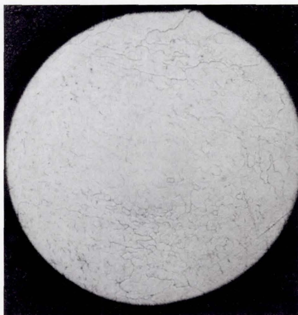
Figure 2.9. Comparison of the microstructure of niobium (Nb) droplets solidified containerlessly. Left—a single grain supercooled about 500 K. Below—multigrain sample that was not supercooled and shows evidence of a shrinkage cavity. (Magnification 20x)
