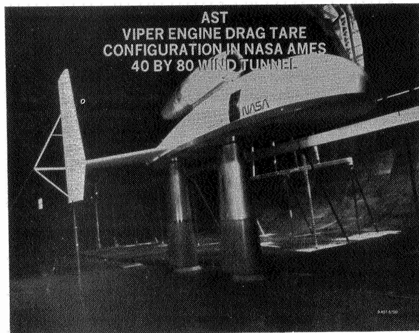
Figure 18.- NASA Ames 40- × 80-ft wind tunnel installation with simulated horizontal tail surface attached.
