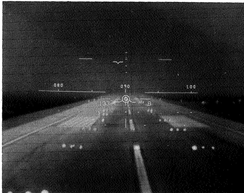
(h) Tracking ground-proximity symbol in flare.
