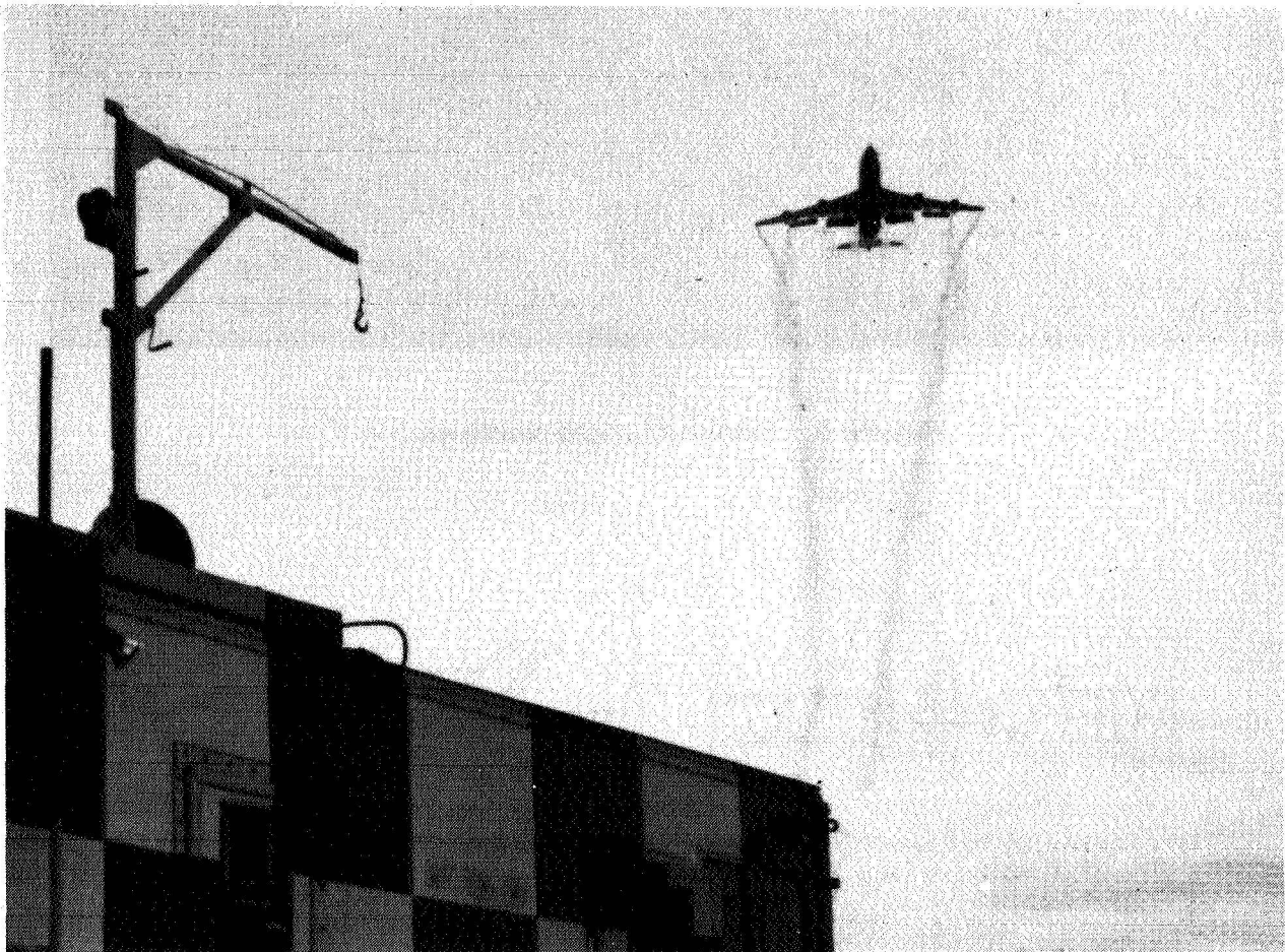
Figure 5. LDV system monitoring wake vortices generated by a B-747 aircraft at Rosamond Dry Lake.
