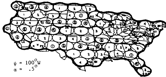
Figure 5 BEAM TOPOLOGY PLAN USING ELLIPTICAL CROSS SECTION COMPONENT BEAMS WITH r = 1.6 MAJOR TO MINOR AXIS RATIO. \alpha_{EW} = .632^\circ , \alpha_{NS} = .375^\circ , n = 64.
