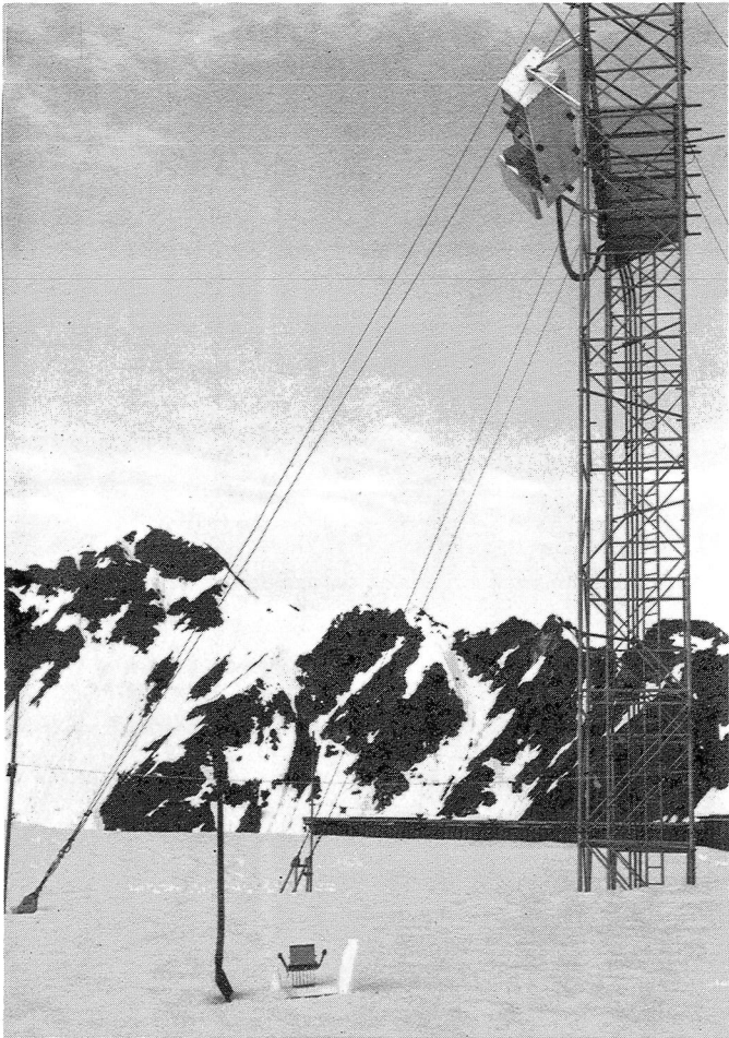
Figure 8 Photo of the test site with radiometer box on the tower, the Ambach snow wetness instrument on the refrozen snow surface in early morning of June 1, 1979.
