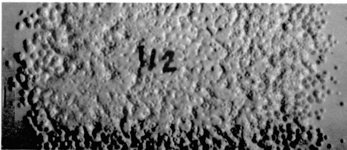
Back of Masonite After Three Hours at 10 V Reverse Bias
