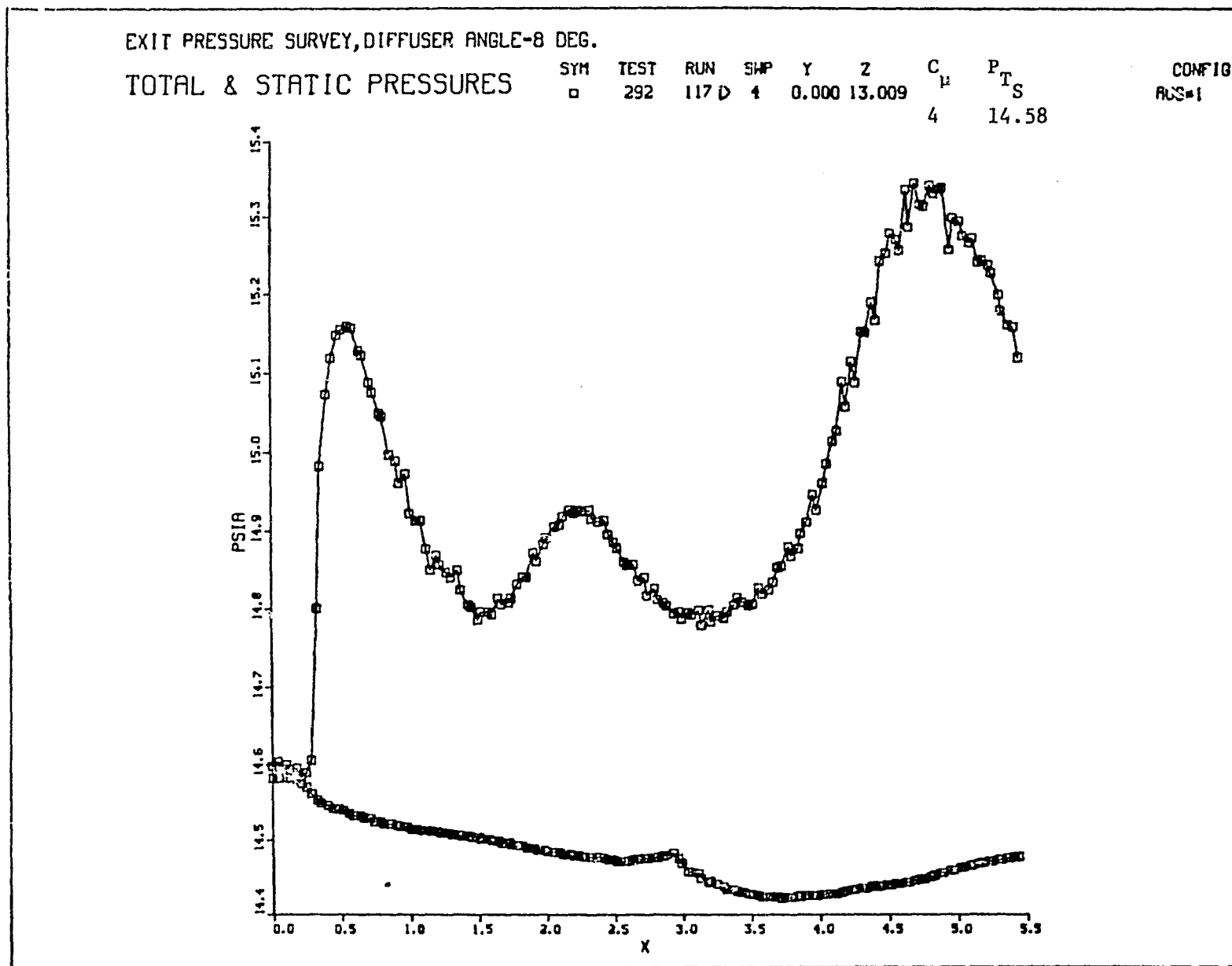
Figure A-9 b. Augmenter Exit Total & Static Pressure, Aug. #1, Diff = 8°, θ = 40°, α = 0
