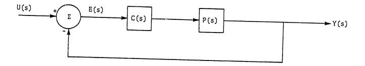
Figure 1. Multivariable feedback control system.
