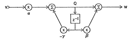
$\begin{bmatrix} z^{-1} \end{bmatrix}$  is a unit time delay of the value Q, in other words, the output of  $\begin{bmatrix} z^{-1} \end{bmatrix}$  is the previous value of Q.
