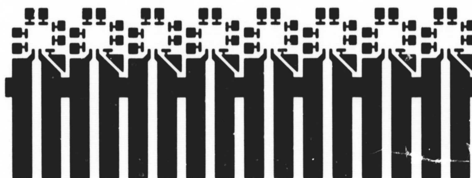
EIGHT-CHIP SUBSTRATE METALLIZATION PATTERN
