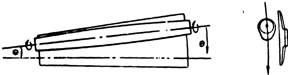
Figure 3-10. Generation of Paraboloidal Contour by Shaped Radial Cutter
