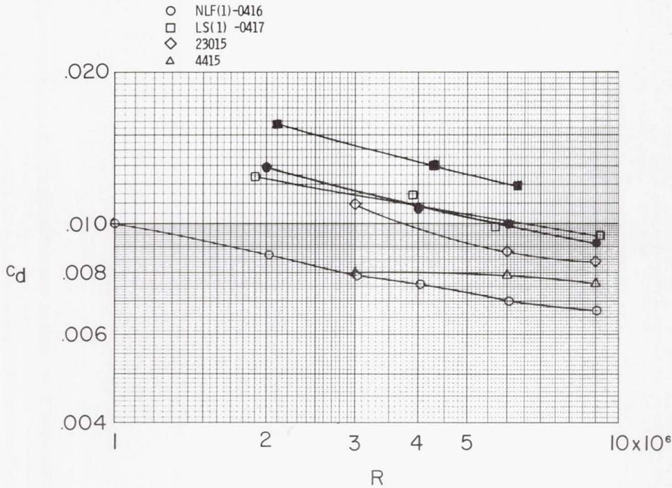
Figure 38.- Comparison of drag coefficients at  $c_l = 1.0$  for NLF(1)-0416, LS(1)-0417, NACA 23015, and NACA 4415 airfoils. Open symbols represent data with transition free; solid symbols, data with transition fixed.
