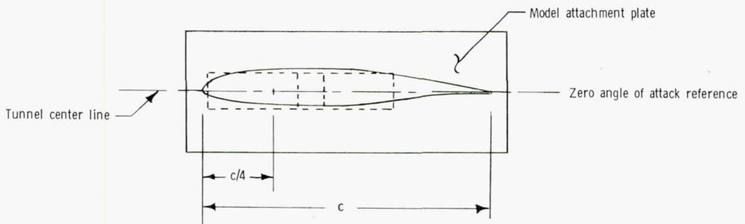
Figure 3.- Typical airfoil model mounted in wind tunnel. All dimensions are in terms of model chord;  $c = 61.0 \text{ cm (24.0 in.)}$ .
