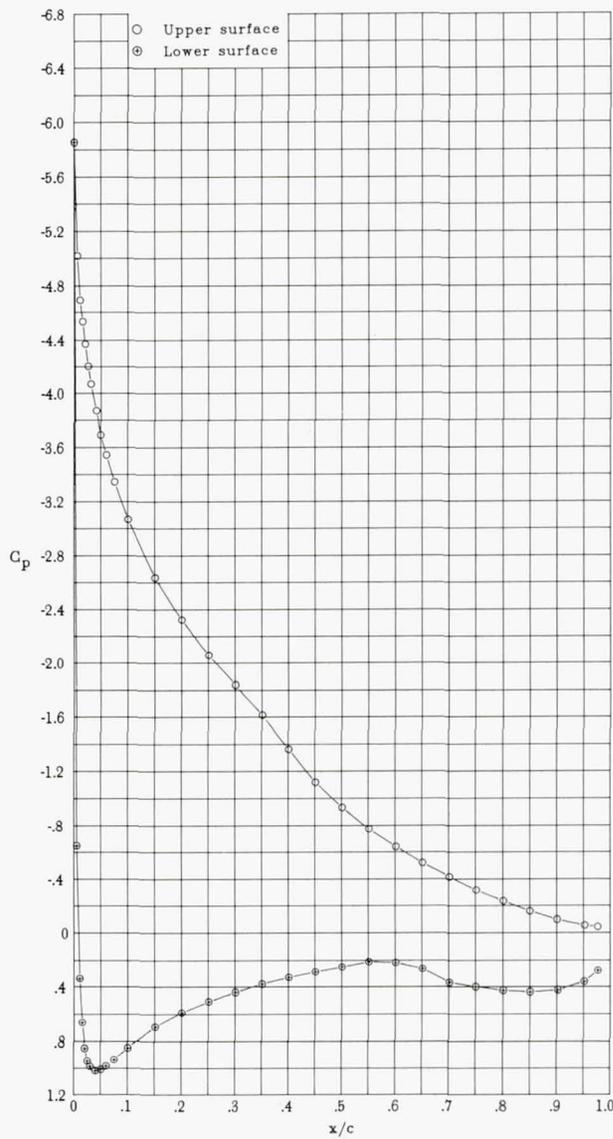
(dd)  $\alpha = 13.24^\circ$ ;  $c_l = 1.731$ ;  $c_d = 0.0212$ ;  $c_m = -0.090$ .
