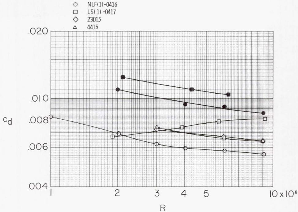
Figure 37.- Comparison of drag coefficients at  $c_l = 0.4$  for NLF(1)-0416, LS(1)-0417, NACA 23015, and NACA 4415 airfoils. Open symbols represent data with transition free; solid symbols, data with transition fixed.
