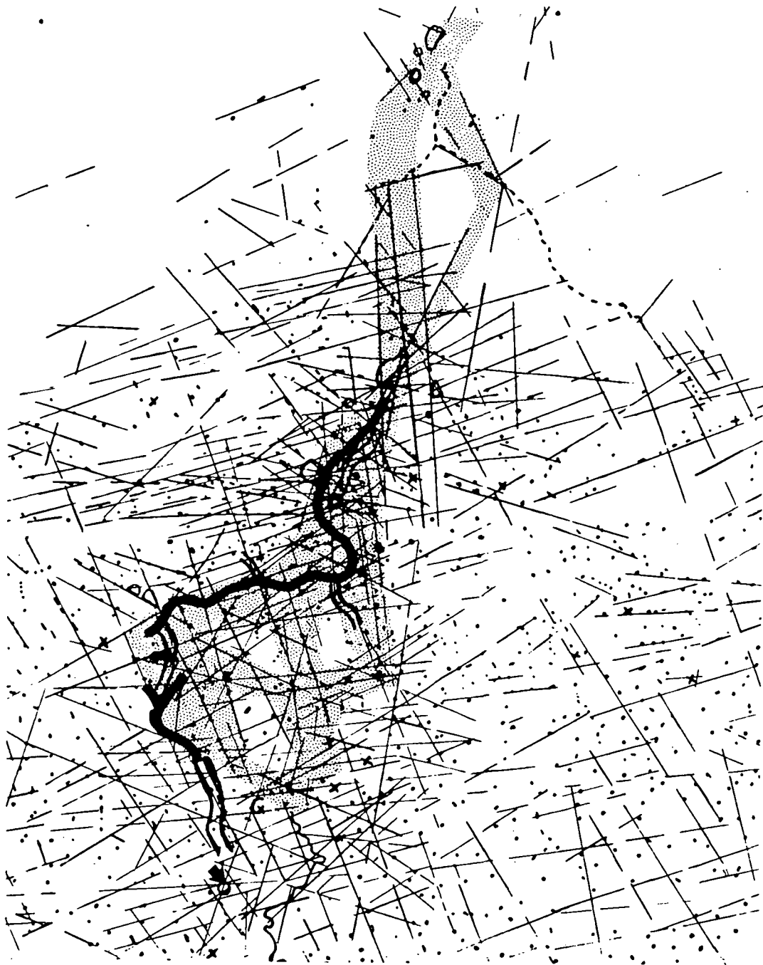
Figure E3 - Map of lineaments and sinkholes in the Camuy Cave area showing the approximate location of the known part of the cave. The agreement with the predicted probable location (gray stippled area) is generally good. (from Rinker).
