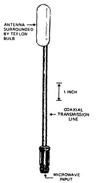
Coaxial applicator designed for operation at 2450 MHz.
