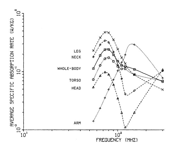
Part-body SAR for homogeneous model of man. Incident intensity = 1 mW.cm<sup>2</sup>.
