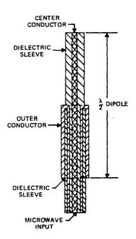
Cross section of the dipole amenna of a coaxial applicator.
