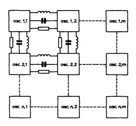
FIG. 45. TWO-DIMENSIONAL COUPLED OSCILLATOR STRUCTURE FOR DIGESTIVE TRACT MODELLING.
