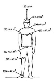
FIG. 26. CALCULATED CURRENT DENSITIES IN A GROUNDED MAN IN RESPONSE TO A 60-HERTZ, 10,000 VOLT/METER ELECTRIC FIELD (FROM KAUNE & PHILLIPS, 1980).
