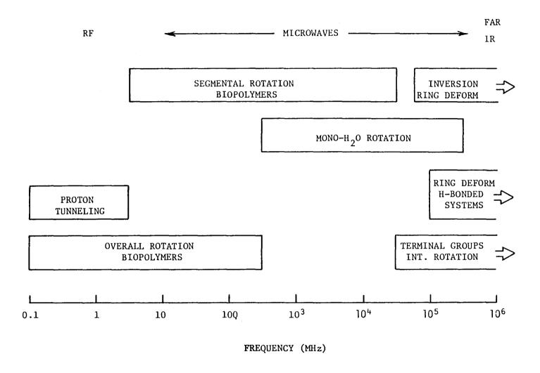
FIG. 41. SOME MOLECULAR RESPONSES TO ELECTROMAGNETIC RADIATION (FROM STUCHLY, 1977).
