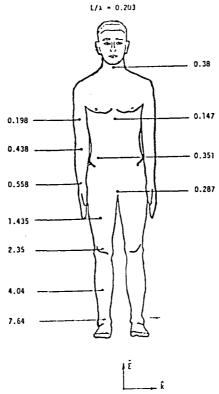
Distribution of power deposition for a human being with feet in electrical contact with the ground. The numbers are relative to whole-body-averaged SAR values of  $(1.75/L_m) \cdot 4.0$  W/kg for 10 mW/cm<sup>2</sup>.
