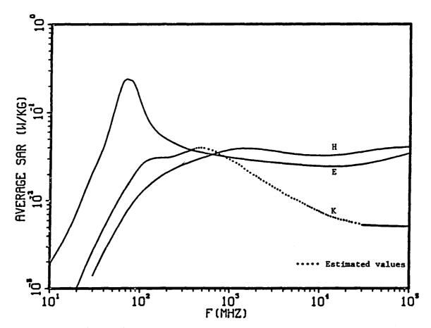
Calculated average SAR in a prolate spheroidal model of an average man for an incident power density of 1  $mW/cm^2$  for three polarizations; a = 0.875 m, b = 0.138 m,  $V = 0.07 m^3$ .
