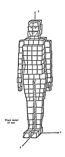
FIG. 22. MULTIPLE CUBE MODEL USED FOR DETAILED SAR COMPUTATIONS (FROM CHATTERJEE ET AL, 1980).
