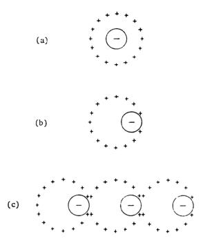
(a) A negatively charged particle (-), together with a double (+) layer, forms an electrically neutral whole; (b) an induced dipole which arises when a charged particle enters an electrical field; (c) linking of oriented dipoles in the direction of an electrical field (chain formation).
