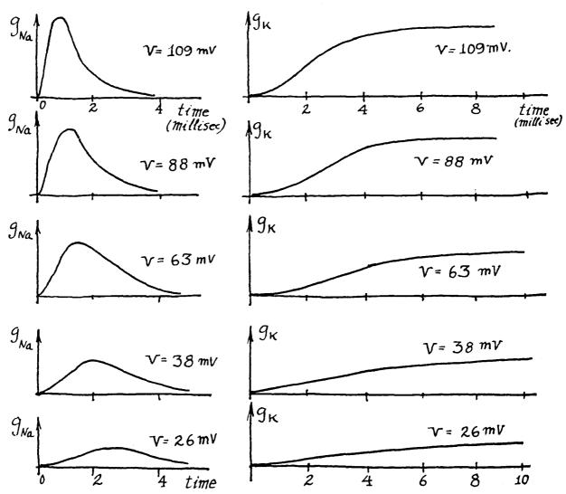
FIG. 3.3-20: TIME COURSE OF SODIUM AND POTASSIUM CONDUCTANCES FOLLOWING A DEPOLARIZATION STEP  $\nu$  AT t=0. CONDUCTANCE UNITS  $10^{-2}/Ohm$  cm². DEPOLARIZATION  $\nu$  IN MILLIVOLTS.
