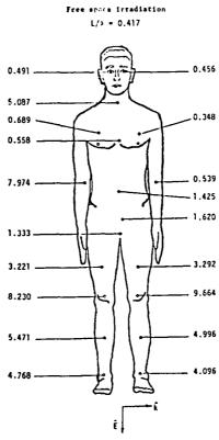
Distribution of power deposition for a human under free-space irradiation. The numbers indicated are relative to whole-body-averaged SAR of  $(1.75/L_m) \cdot 1.88$  W/kg for 10 mW/cm<sup>2</sup> incident fields.
