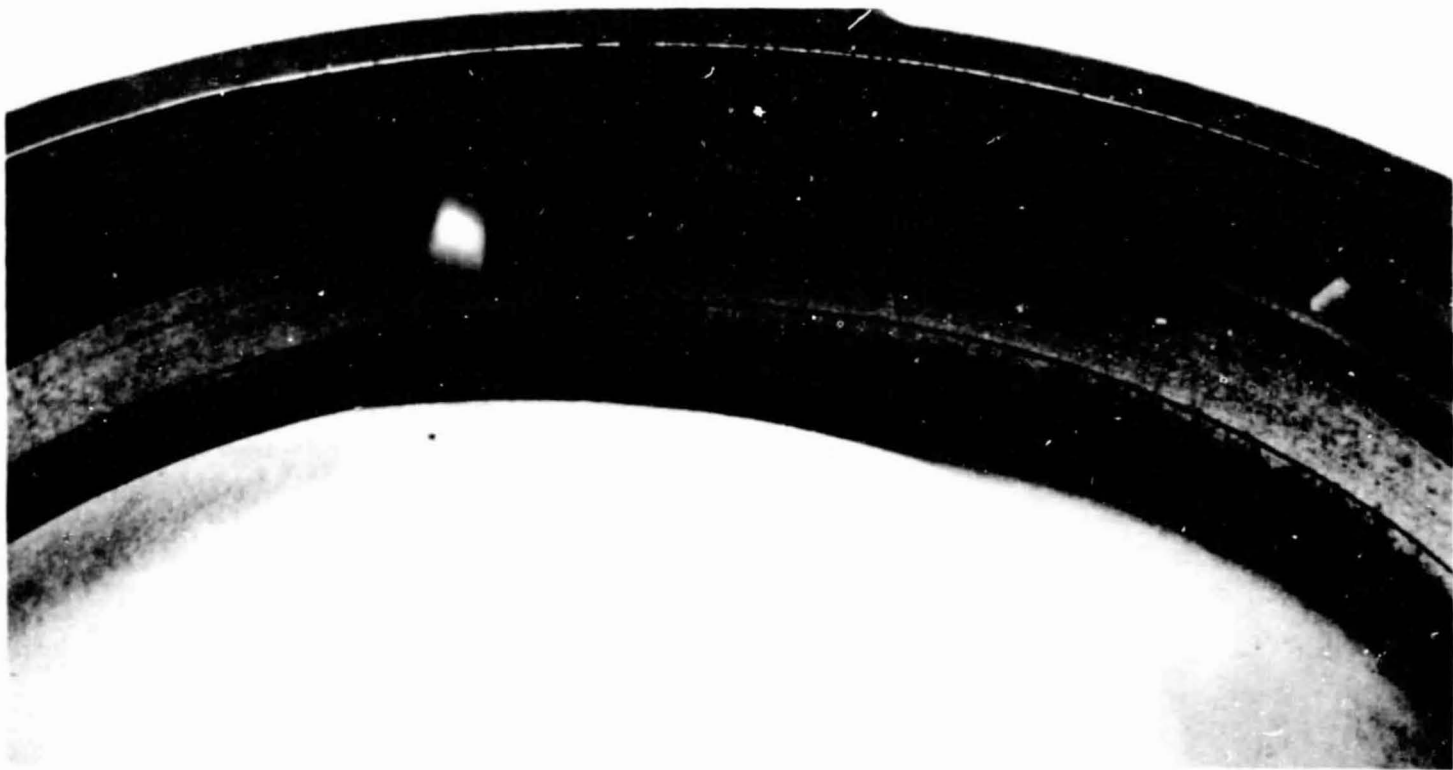
Figure 98. Pump End Primary Seal Ring (Position 2), P/N 7R0011525, S/N 047909, Build 15, Posttest 297
