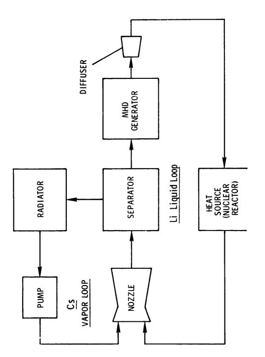
Fig. 1 Liquid-metal MHD system proposed by Elliott (Reference 2).
