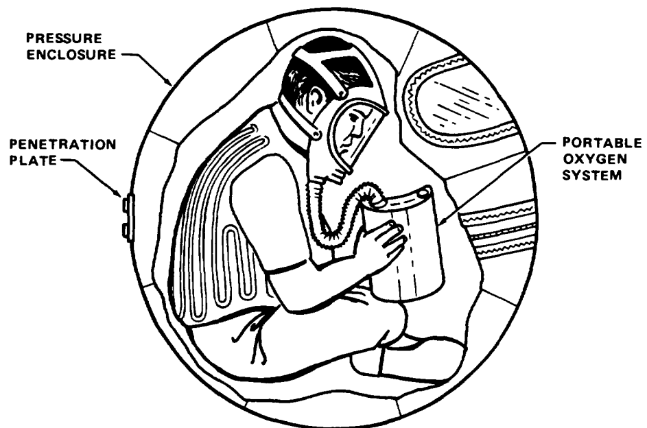
Figure 5-19.—Personal rescue system.
