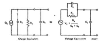
Equivalent circuits of piezoelectric accelerometer with connection cable
