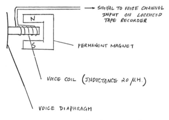
FIGURE 2. Schematic for voice microphone of the tape recorder.
