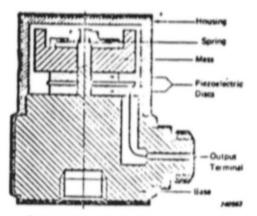
Schematic of piezoelectric accelerometer
