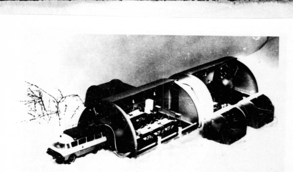
Figure 6 - Model of the field laboratory set up at the spacecraft recovery site. Electric generators and environmental control equipment provide the necessary conditions for the initial observation and examinations of biological specimens.
