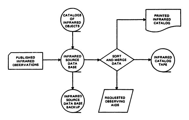
Figure 1. Flow chart of Infrared Catalog and Data Base
