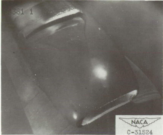
(a) Alternate door 20 percent open; preheat-air inlet temperature, 204° F; carburetor top-deck mass air flow, 2.1 pounds per second.
