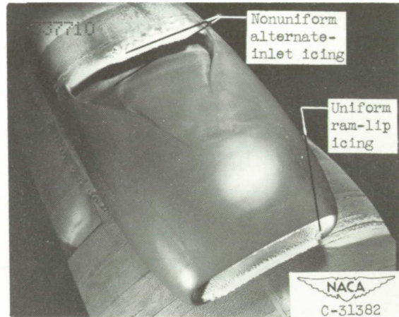
(b) Ice formed after 25 minutes of icing. Tunnel-air total temperature, 25° F; mass-flow ratio, 0.7.
