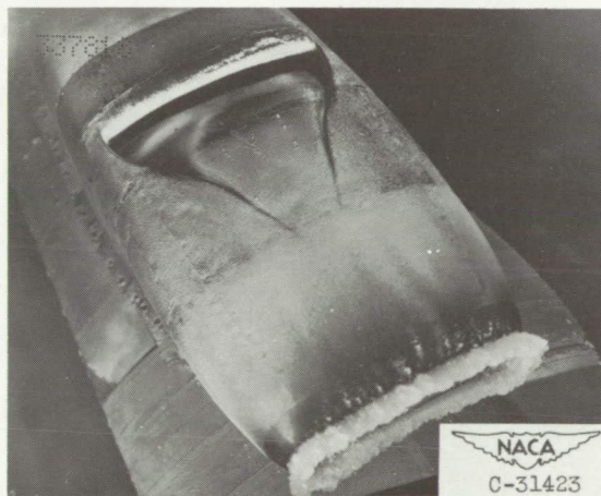
(c) Liquid-water content, 1.6 grams per cubic meter; median droplet diameter, 21 microns; icing time, 15 minutes.
