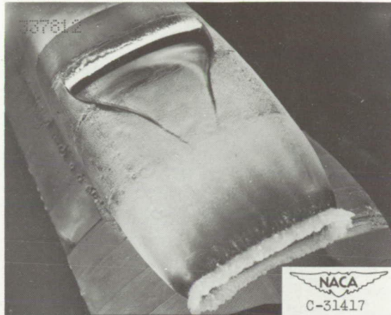
(b) Liquid-water content, 1.5 grams per cubic meter; median droplet diameter, 20.5 microns; icing time, 15 minutes.
