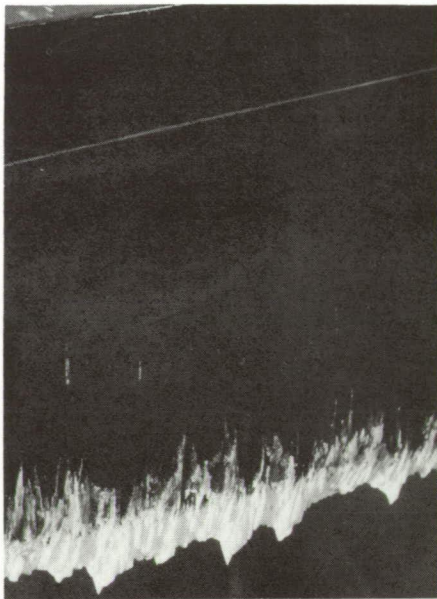
(b) Boot B after 6 minutes in icing.
