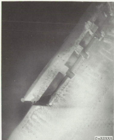
Lower surface. Icing time, 7\frac{1}{2} minutes; before ice removal.
