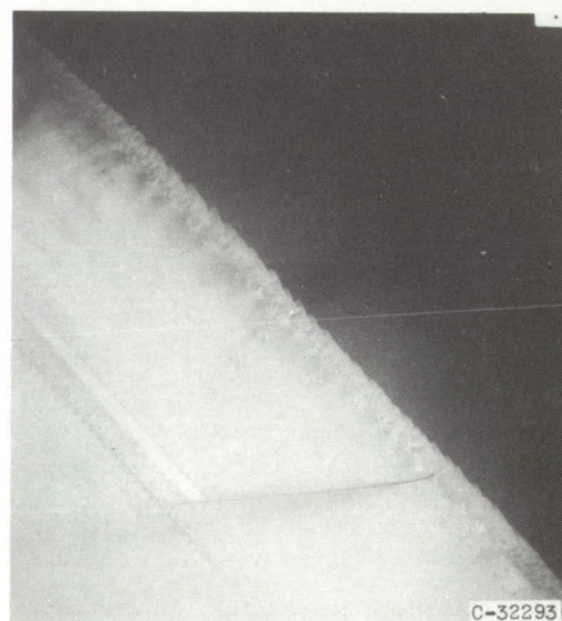
Upper surface. Icing time, 10\frac{1}{2} minutes; section drag coefficient, 0.0260.
