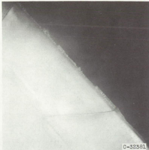
Upper surface. Icing time, 7\frac{1}{2} minutes; section drag coefficient, 0.0280.
