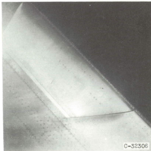
Upper surface. Icing time, 2\frac{1}{2} minutes; section drag coefficient, 0.0187.
