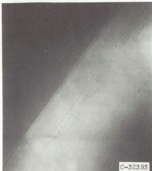
Lower surface. Icing time, 4\frac{1}{2} minutes; section drag coefficient, 0.0101.
