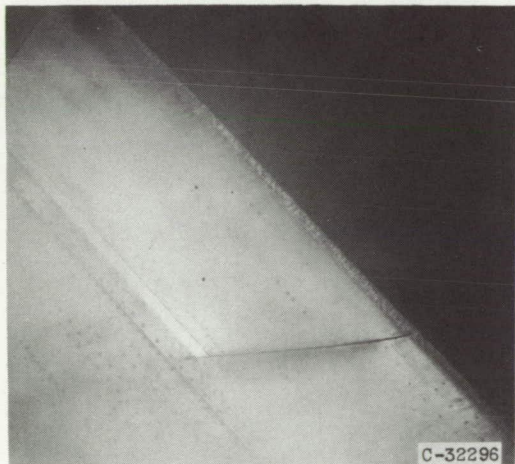
Upper surface. Icing time, 4\frac{1}{2} minutes; section drag coefficient, 0.0180.
