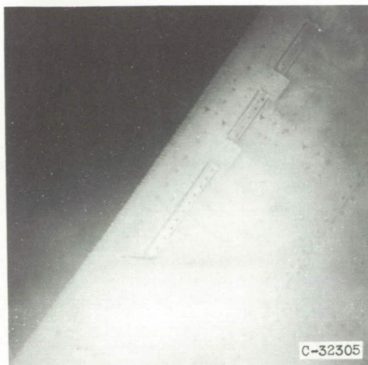
Lower surface. Icing time, 2 minutes; section drag coefficient, 0.0177.
