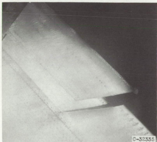
Upper surface. Icing time, 11 minutes; section drag coefficient, 0.0417; before ice removal.
