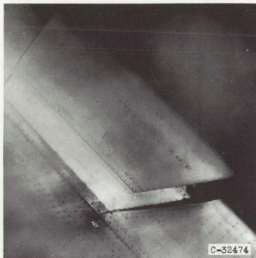
Upper surface. Icing time, 13 minutes; section drag coefficient, 0.0386.
