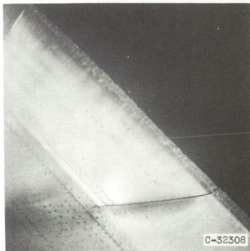
Upper surface. Icing time, 5\frac{1}{2} minutes; section drag coefficient, 0.0239.
