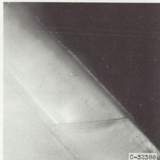
Upper surface. Icing time, 12 minutes; section drag coefficient, 0.0155.
