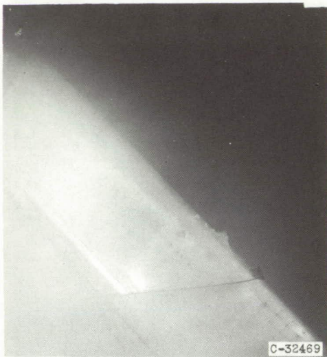
Upper surface. Icing time, 33 minutes; section drag coefficient, 0.0117.
