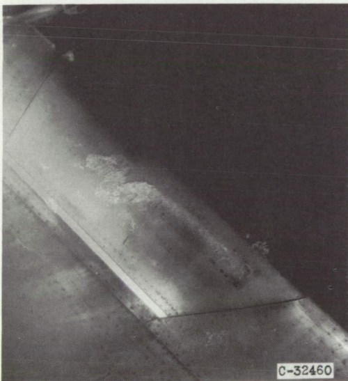
Upper surface. Icing time, 59 minutes; section drag coefficient, 0.0140.
