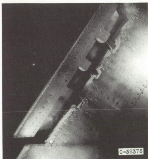
Lower surface. Icing time, 10 minutes; section drag coefficient, 0.0329.
