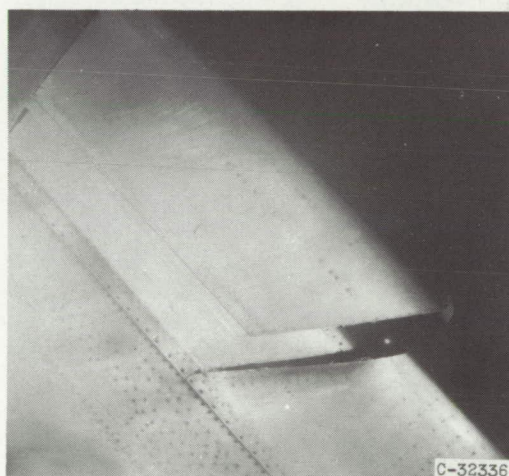
Upper surface. Icing time, 11\frac{1}{2} minutes; section drag coefficient, 0.0383; after ice removal.
