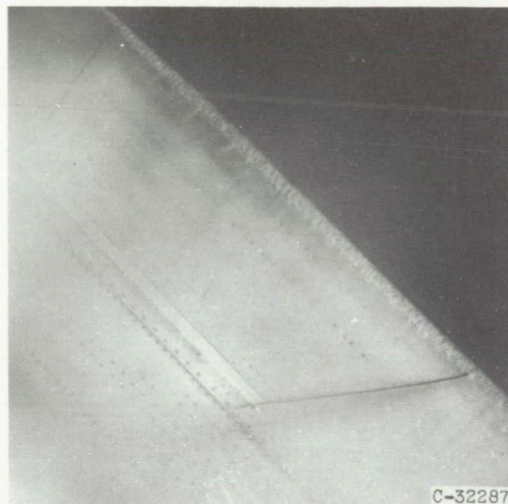
Upper surface. Icing time, 5\frac{1}{2} minutes; section drag coefficient, 0.0177.
