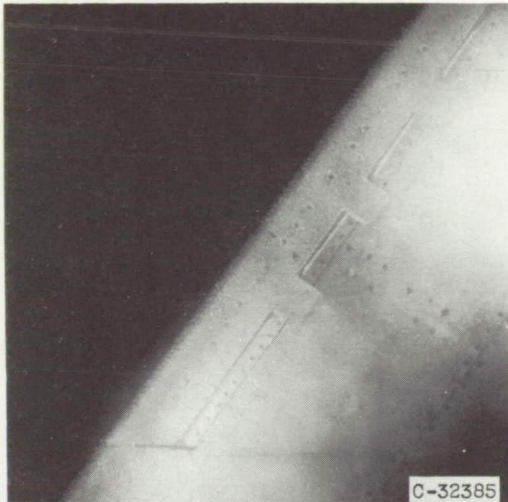
Lower surface. Icing time, 4 minutes; section drag coefficient, 0.0112.
