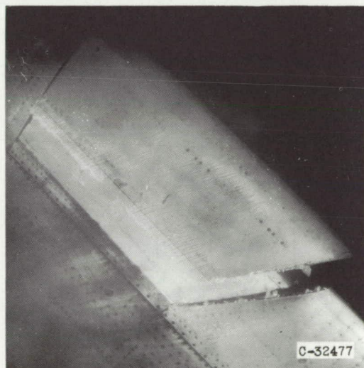
Upper surface. Icing time, 33 minutes; section drag coefficient, 0.0434.
