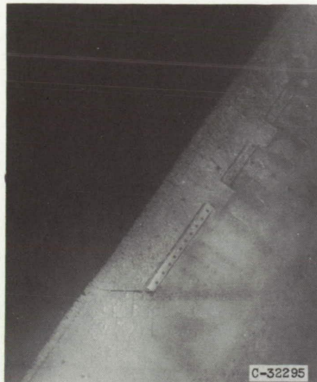
Lower surface. Icing time, 2\frac{1}{2} minutes; section drag coefficient, 0.0136.
