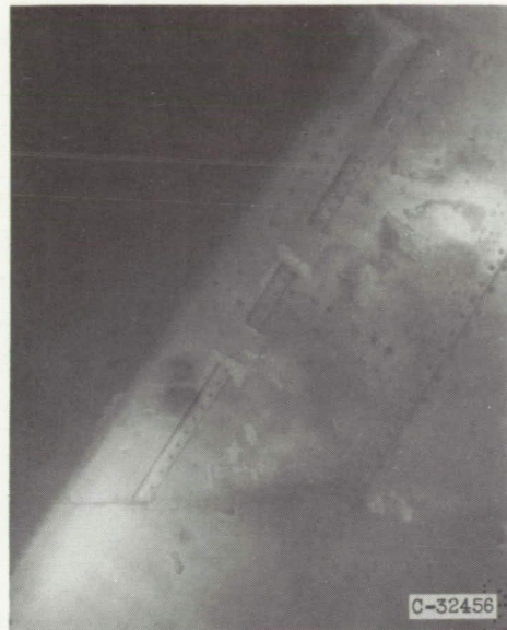
Lower surface. Icing time, 43\frac{1}{2} minutes; section drag coefficient, 0.0094.
