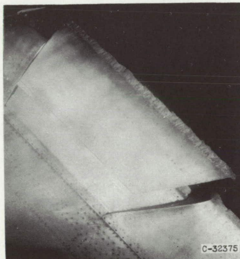
Upper surface. Icing time, 11 minutes; section drag coefficient, 0.0576.
