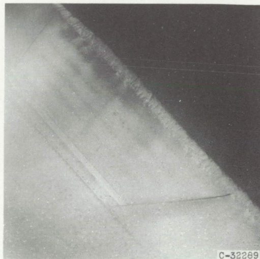
Upper surface. Icing time, 10\frac{1}{2} minutes; section drag coefficient, 0.0265.
