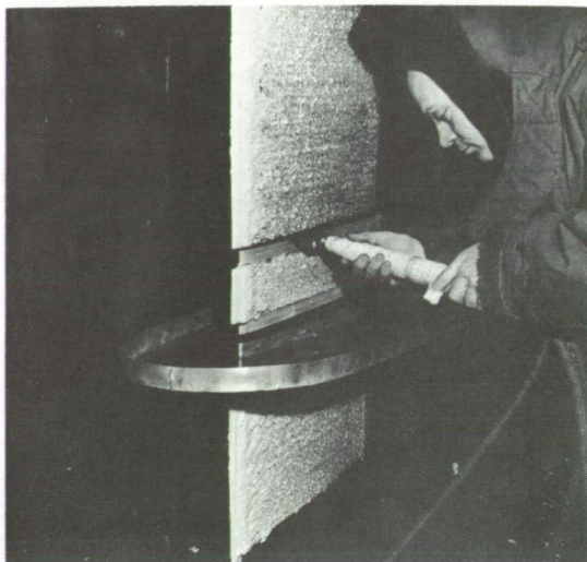
(d) Removal of ice with heated ice scraper prior to weighing.
