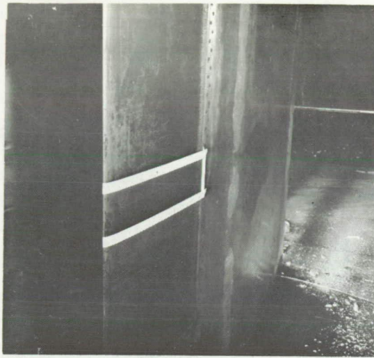
(a) Celluloid sheet installed prior to icing exposure.
