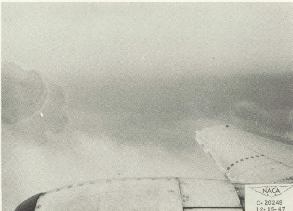
Figure 12. - Formation of ice on outboard-wing panel showing sections of ice lost by wing flexure. Average icing rate, 4 inches per hour; liquid-water content, 0.4 gram per cubic meter; droplet size, 17 microns. (Painted stripes are 1 in. wide.)
