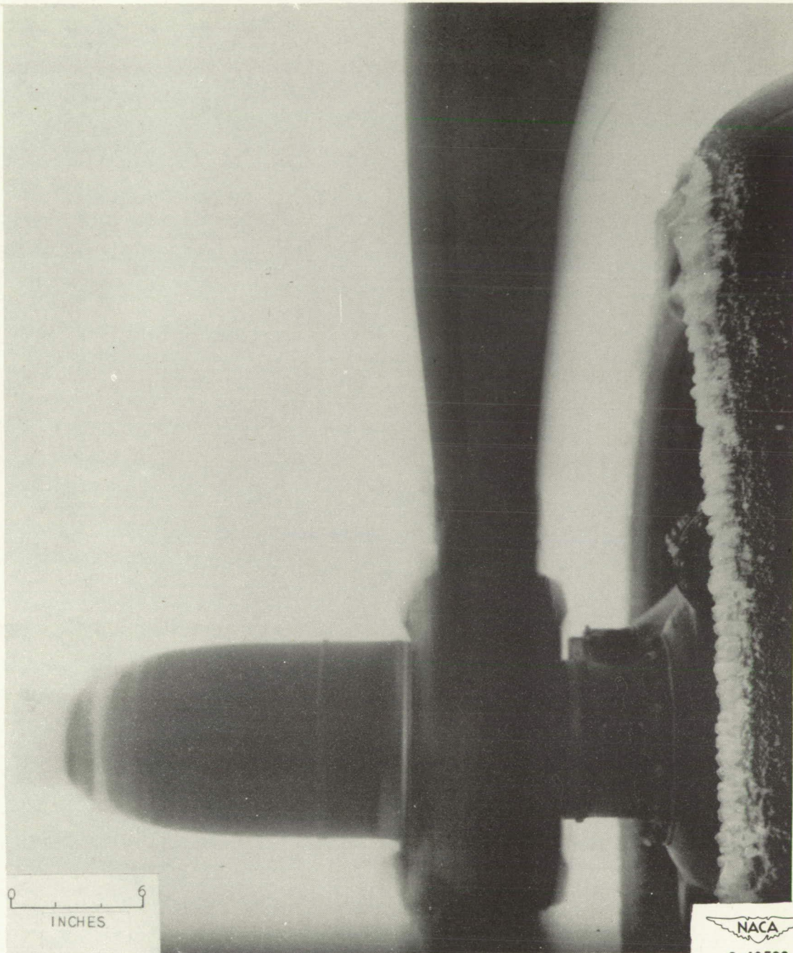
Figure 10. - Formation of ice on leading edge of cowl and spinner. Average icing rate, 4 inches per hour; liquid-water content, 0.4 gram per cubic meter; droplet size, 17 microns.
