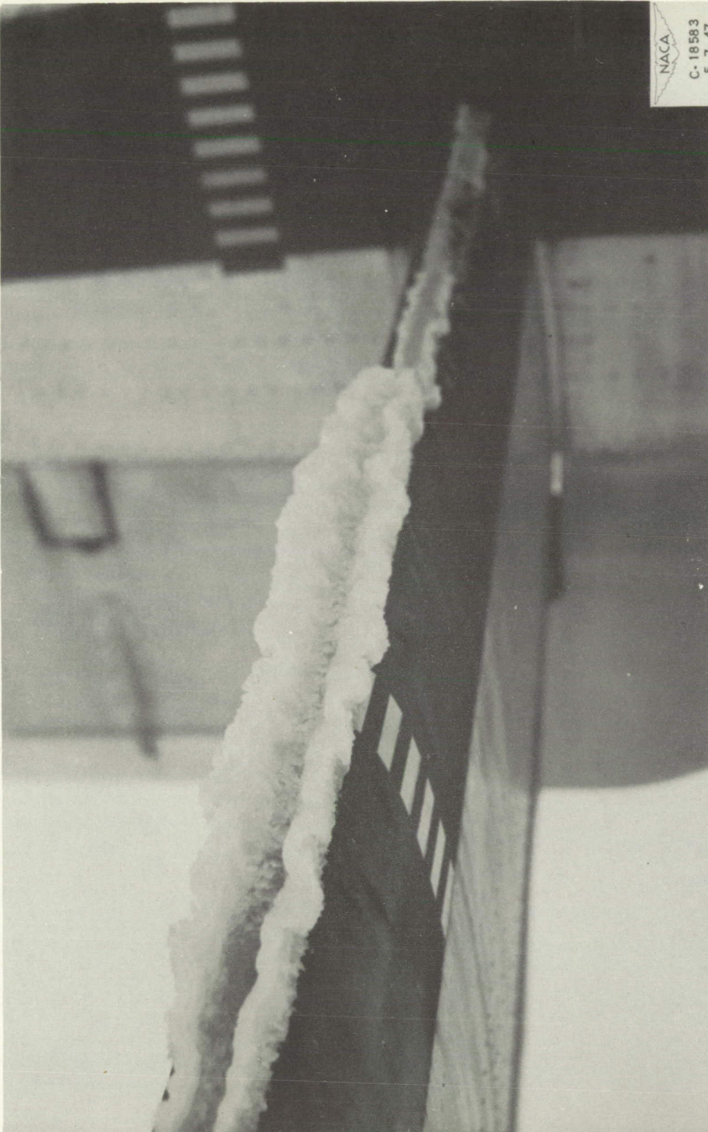
Figure 13. - Formation of ice on horizontal stabilizer. Average icing rate, 4 inches per hour; liquid-water content, 0.4 gram per cubic meter; droplet size, 17 microns. (Painted stripes are 1 in. wide.)
