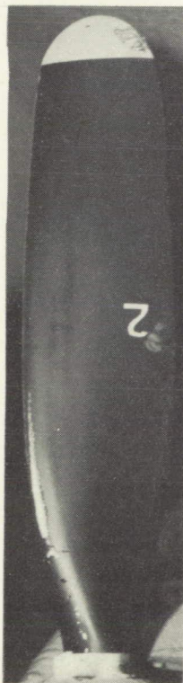
(e) Heating rate, 31,900 Btu per hour per blade; tunnel-air temperature, -2^{\circ} F.
