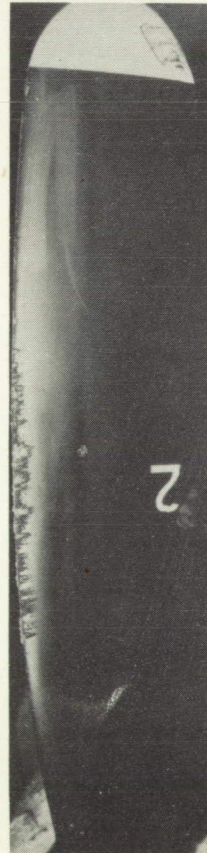
(a) Heating rate, 31,000 Btu per hour per blade; tunnel-air temperature, 17° F.
