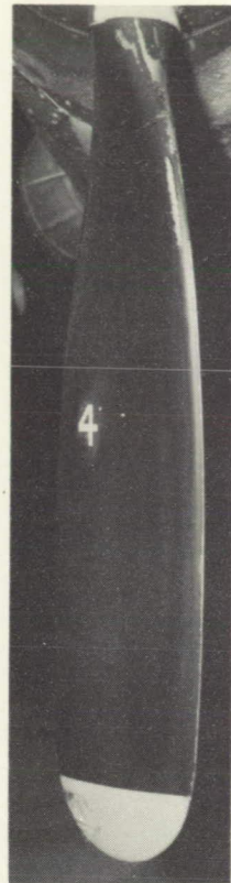
(f) Heating rate, 40,000 Btu per hour per blade; tunnel-air temperature, -2^{\circ} F.
