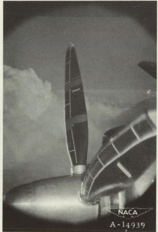
Figure 19.— Ice formation of encounter 2. Camber face. Peak efficiency loss, 1 to 2 percent.
