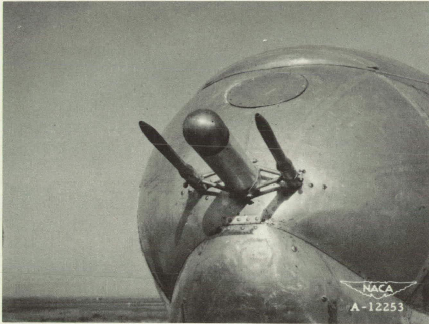
Figure 6.— Hemispherical differential-pressure type yaw and pitch head. Airspeed total-pressure heads are mounted on either side of the yaw and pitch head.
