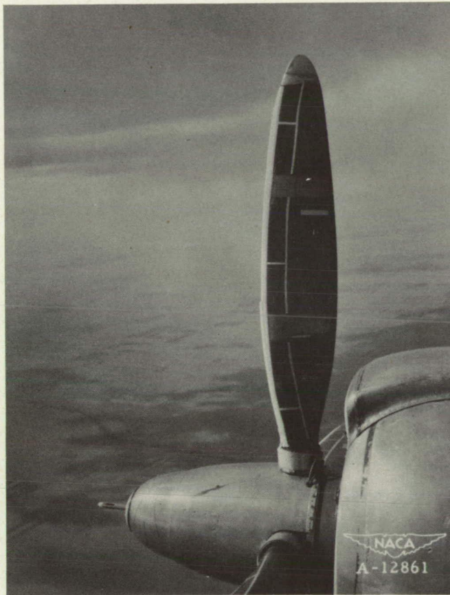
Figure 31.— Ice formation of encounter 12. Camber face. Efficiency loss, 5 percent.
