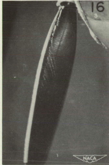
Figure 29.— Ice formation of encounter 10. Thrust face. Efficiency loss, 0 percent.
