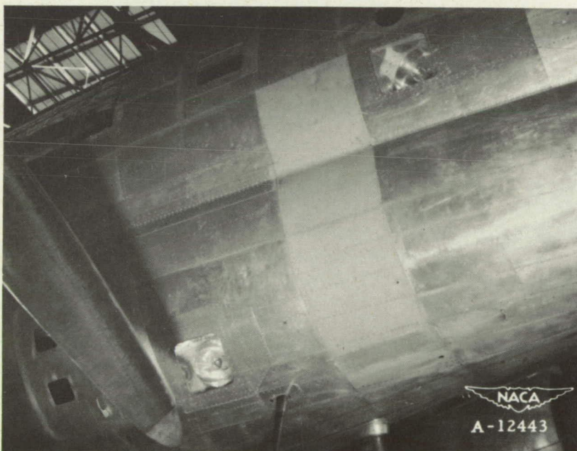
Figure 5.- Propeller camera-flash-lamp installations.
