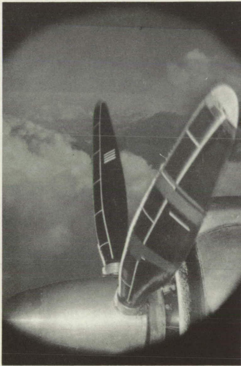
Figure 19.— Ice formation of encounter 2. Camber face. Peak efficiency loss, 1 to 2 percent.
