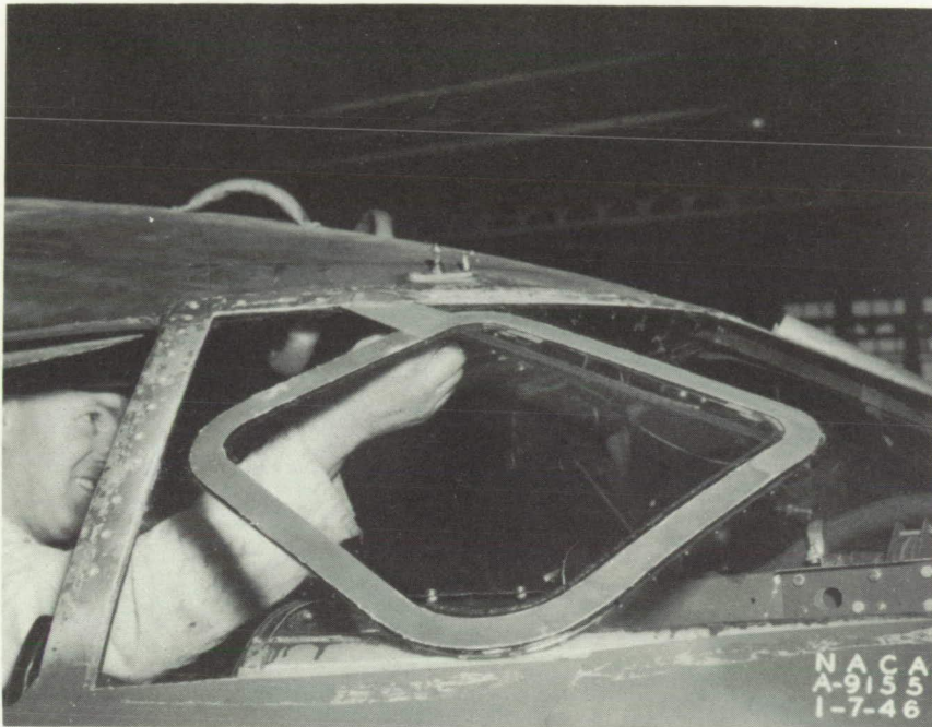
Figure 4.- Electrically heated flush windshield panel, viewed from the exterior of the C-46 airplane cockpit.
