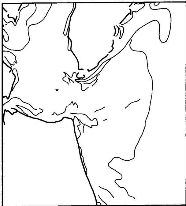
Figure 3a. Visually discriminated turbidity boundaries for Landsat image of 8 July 1978.
