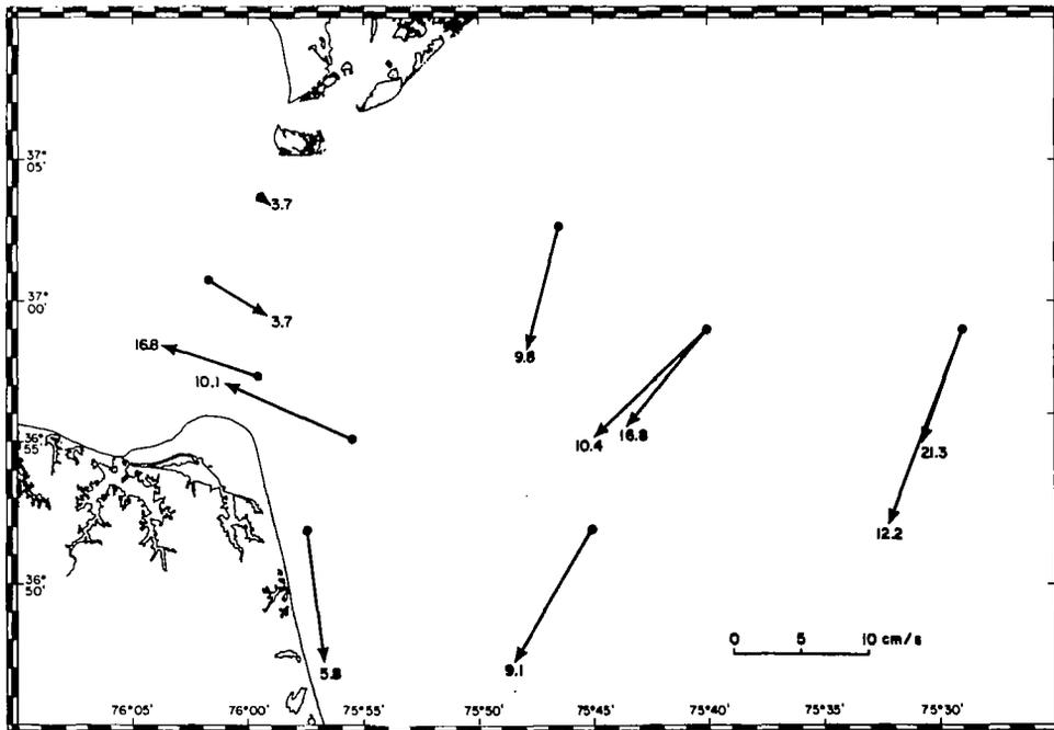
Figure 10.- Mean velocities for 240-hour interval beginning 0000 on 4 February 1979. Depths of measurements (m) are indicated at the head of the velocity arrows. Mooring position designations are shown in figure 9.
