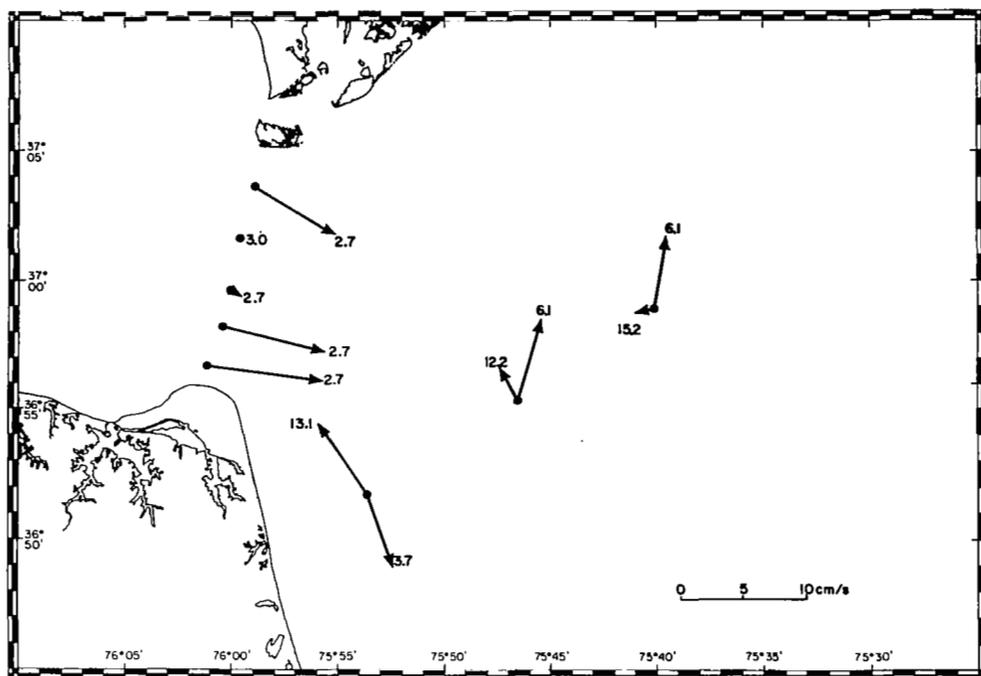
Figure 13.- Mean velocities for 38-day interval beginning 23 June 1980. Depths of measurements (m) are indicated near head of velocity arrows.
